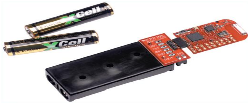
Figura 4.8 - Nodo sensor: eZ430-RF2500T® battery board (Texas Instruments).
