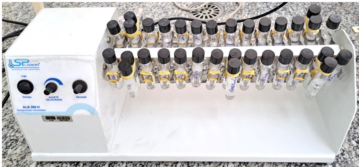
Figure 11. ALB 260 H tube homogenizer loaded with samples during adsorption experiment
