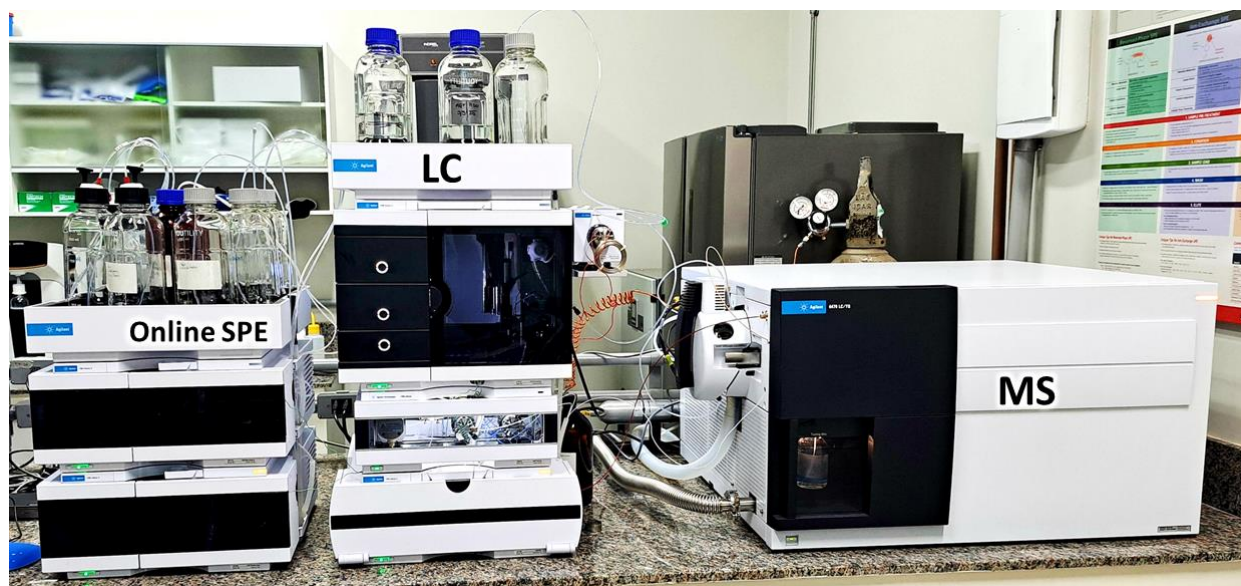
Figure 12. Agilent 1290 Infinity II liquid chromatograph coupled to Agilent 6470B mass spectrometer, equipped with QqQ and ESI
