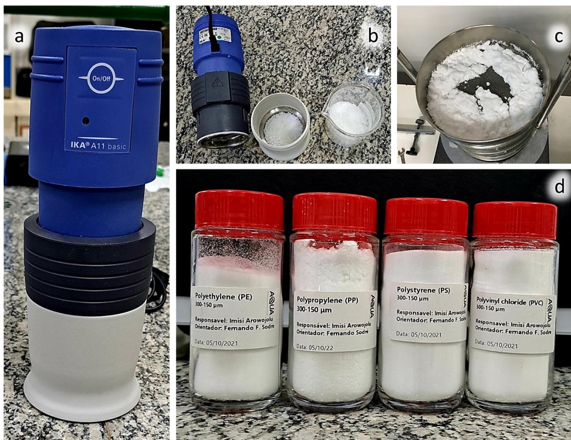
Figure 8. MPs milling materials and stages(a) Cryogenic miller, (b) loading of polymer resin into the milling cup up to the mark, (c) sieving of milled MPs and (d) MPs samples used in this work
