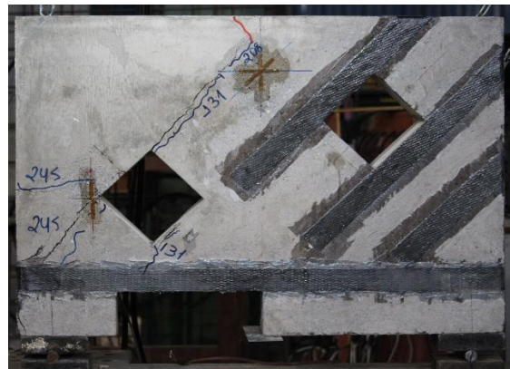
Figura 4.30 – Modo ruptura DB3-H2-S-FS-1
