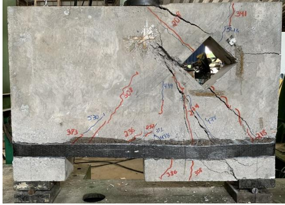
Figura 4.28 – Modo ruptura DB3-W-H1-S-F-1
