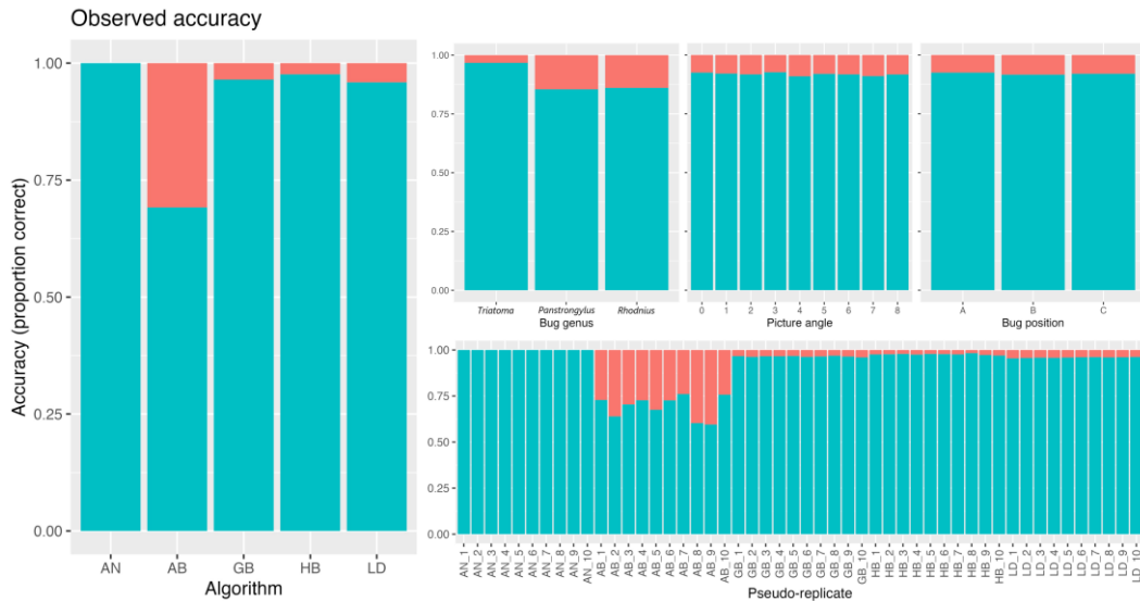
Fig. 2. Cellphone picture-based automated identification of Chagas disease vectors: observed accuracy, measured as the proportion of pictures that were correctly identified (blue bars) to the genus level. Left: results stratified by algorithm (AN, AlexNet; AB, AdaBoost Adaptive Boosting; GB, Gradient Boosting; HB, Histogram-based Gradient Boosting; and LD, Linear Discriminant model). Right, top row: results stratified by (i) triatomine-bug genus, which can be interpreted as sensitivity (the probability of correct identification, conditioned on genus); (ii) the nine angles at which bugs were pictured (see Fig. 1); and (iii) bug position (A, dorsal-flat; B, dorsal-oblique; C, front/back-oblique; see Fig. 1). Bottom-right: results for each of the 10 (pseudo-)replicate runs completed by each algorithm. The data underlying these graphs, along with score 95% confidence intervals for each proportion, are provided in Supplementary Tables S1–S5.
