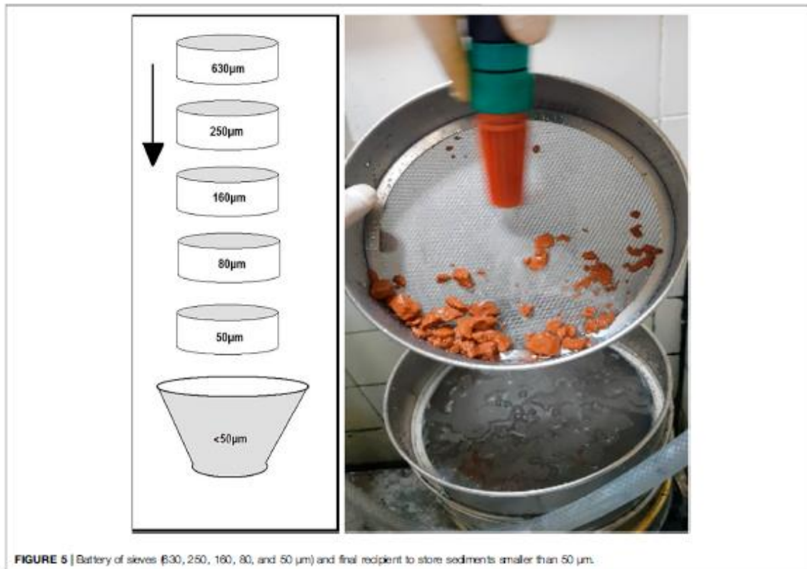
FIGURE 5 | Battery of sieves (630, 250, 160, 80, and 50 \mu\text{m} ) and final recipient to store sediments smaller than 50 \mu\text{m} .
