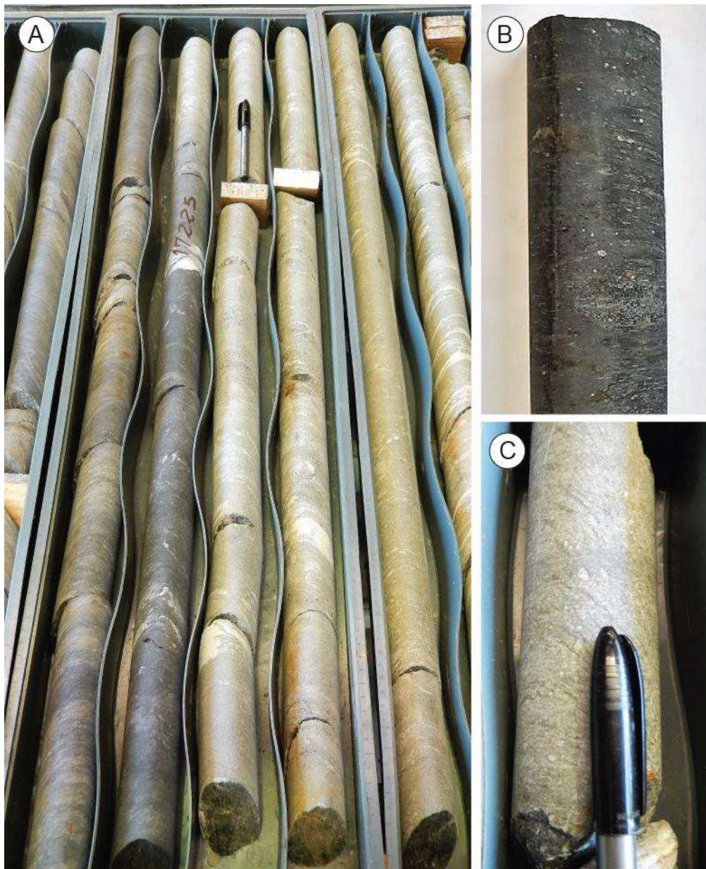
Fig. 4. Drill core aspects of metasedimentary rocks of the Crixás greenstone belt. (A) Transition from black-colored carbonaceous phyllites to light brown-colored metagraywackes (increasing depth from left to right). (B) Highly foliated carbonaceous phyllite. (C) Metagraywacke with white angular clasts of quartz and feldspar.
