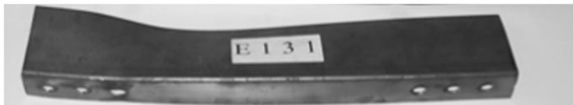
Figura 6.90 – Cantoneira E131 deformada experimental.
