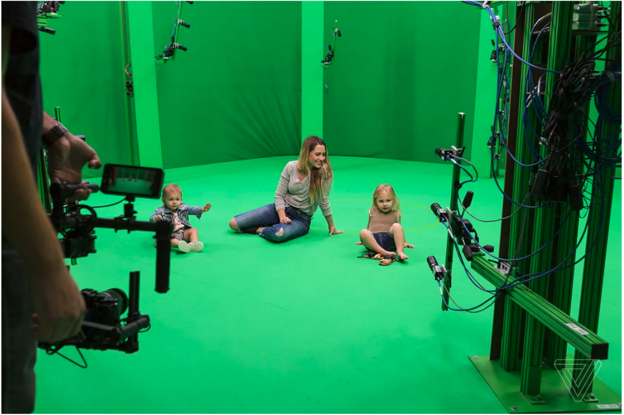
Figure 2.4: Array of cameras for point cloud acquisition at 8i [12].
