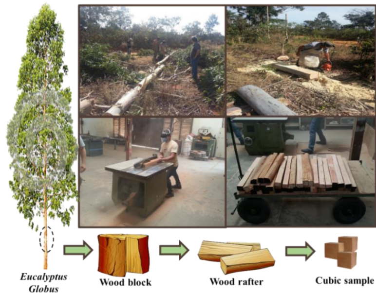
Figure 20. Wood sample confection of a 15-year-old species of Eucalyptus Grandis . Preparation of rafters in the LPF's carpentry.
