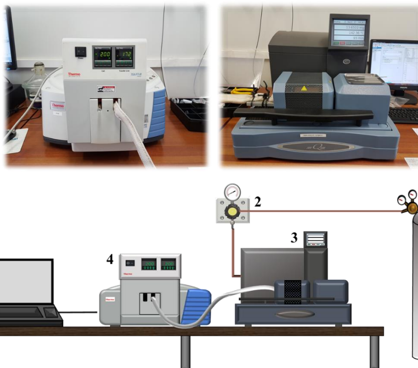
Figure 21. General scheme of the experimental system. 1) N 2 cylinder, 2) Gas control rotameter, 3) SDT Q600 TA, 4) THERMO SCIENTIFIC TGA / FTIR, 5) Computer (OMNIC and Qseries Software).
