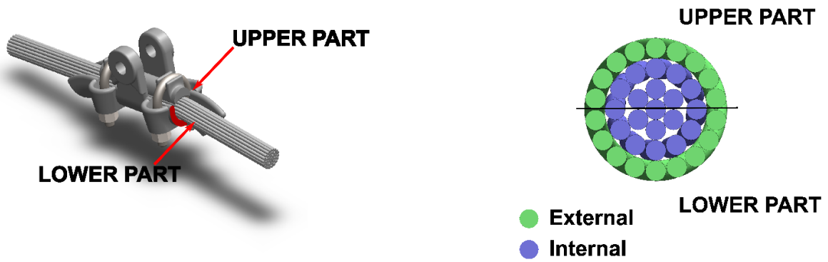
Fig. 3.3. Terminology for the identification of the location of wire breaks within the cross section of the AAAC 900 MCM conductor.
