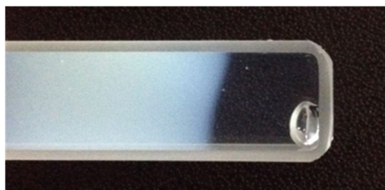
Figure 5. Air bubble in an irradiated modified VIPARnd gel cuvette.
