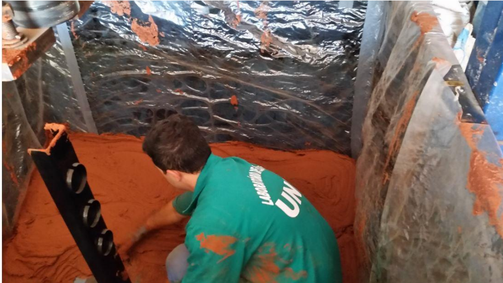
Figure 3.14. Placing the soft soil into the box.
