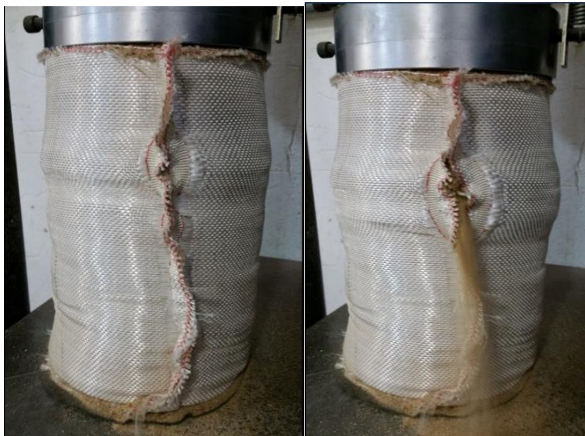
Figure 3.30. Failure of the small columns due to loading at seam.
