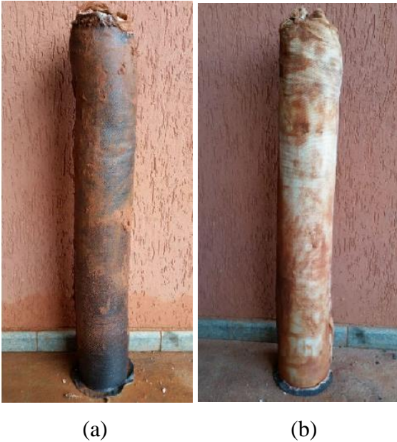
Figure 4.3. Encased column after loading test: (a) G-2 and (b) G-1.
