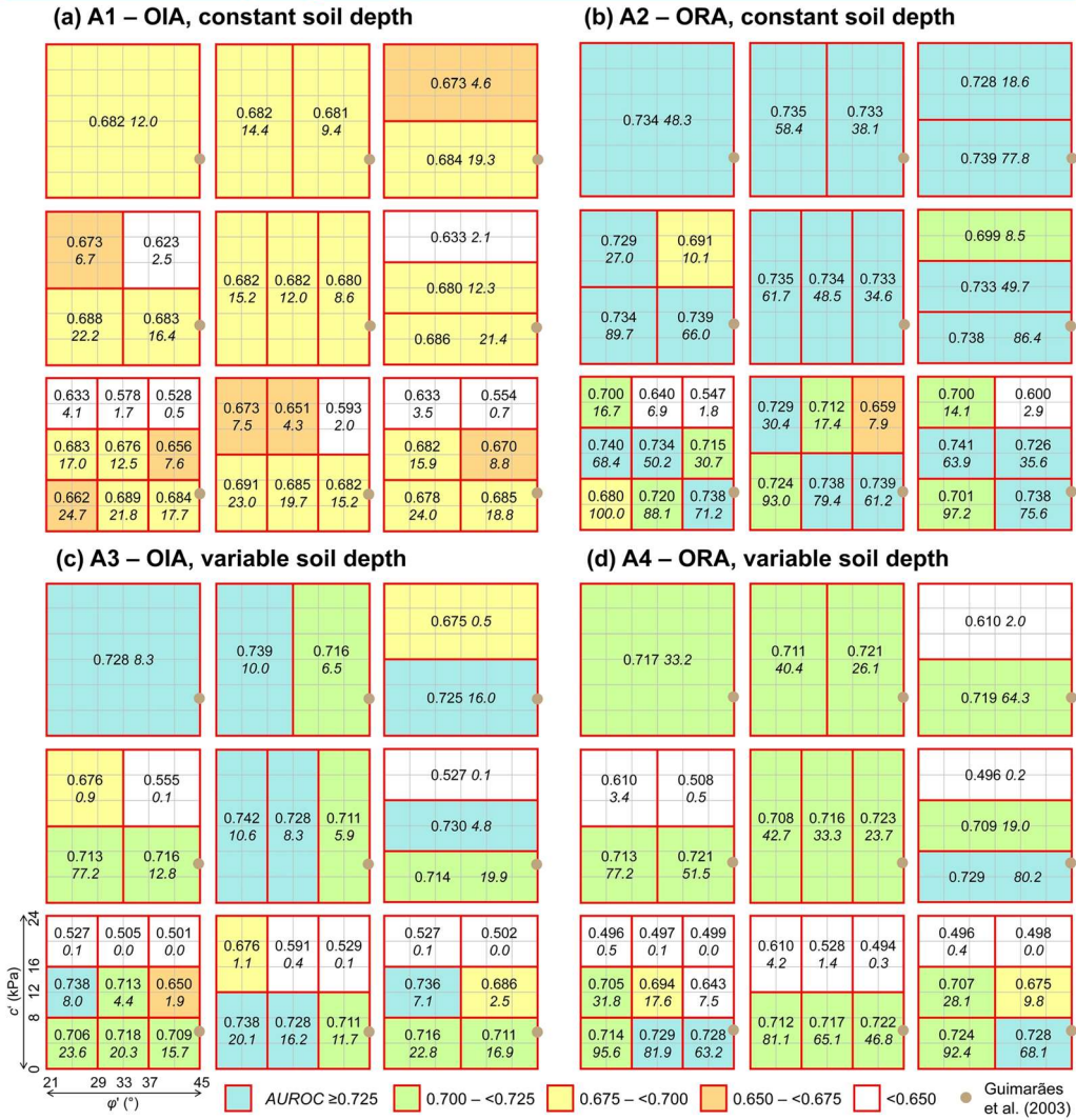
Fig. 5 Results of tests A1–A4 in terms of model performance ( AUROC ) and factor of conservativeness ( FoC , in italic letters ). See Fig. 3 for the configuration of the parameter space
