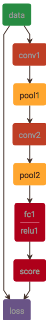
Figure 5.8: Variant of the LeNet (LECUN et al., 1989) as a Directed Acyclic Graph
