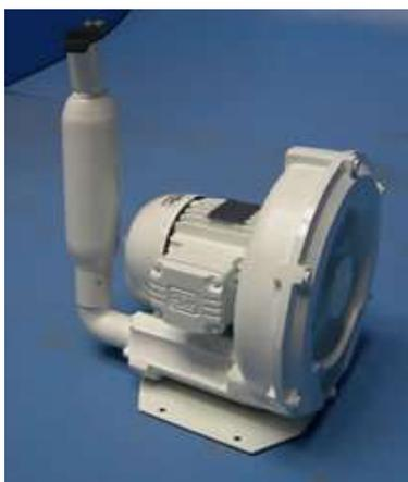
Figura A.7 – Compressor Radial CR-2.
