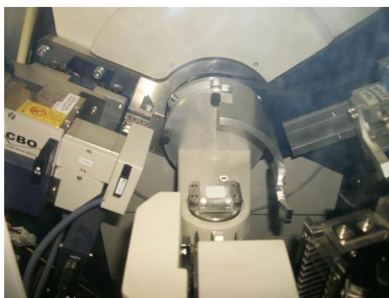
Figura 3.8 - Difratormetro de raios X (DRX), Ultima IV X-ray diffractometer, Rigaku .
