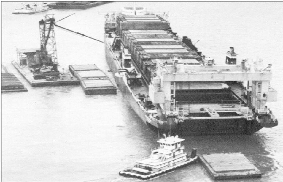
**Figura 4.2.1:** Navio Lighter Aboard Ship (Lash)
