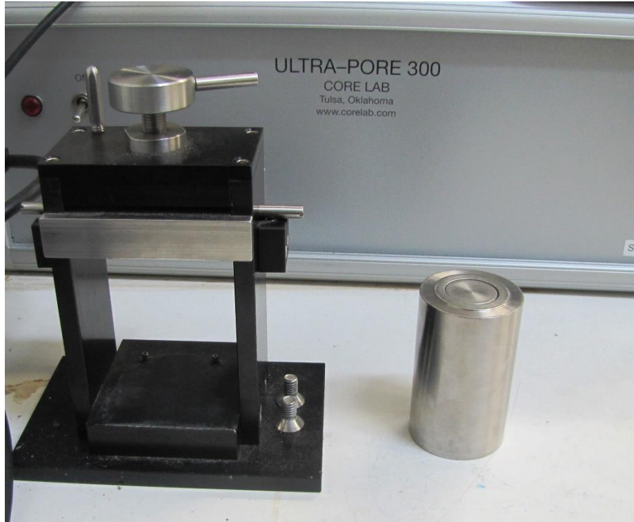
Figure 3.7. Ultra-Pore 300 Porosimeter with matrix cup and analysis plugs
