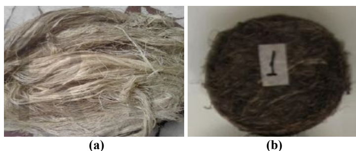
Figura 31 - Bananeira: (a) fibra (BHATNAGAR et al. , 2015) (b) Amostra 2A confeccionada com a fibra (DEMARCHI, 2010).
