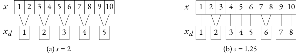
Figure 3.2: Illustration of the downsampling process in a 1D voxelized structure. Parent nodes ( x_d ) serve as hierarchical representatives of child nodes ( x ).
