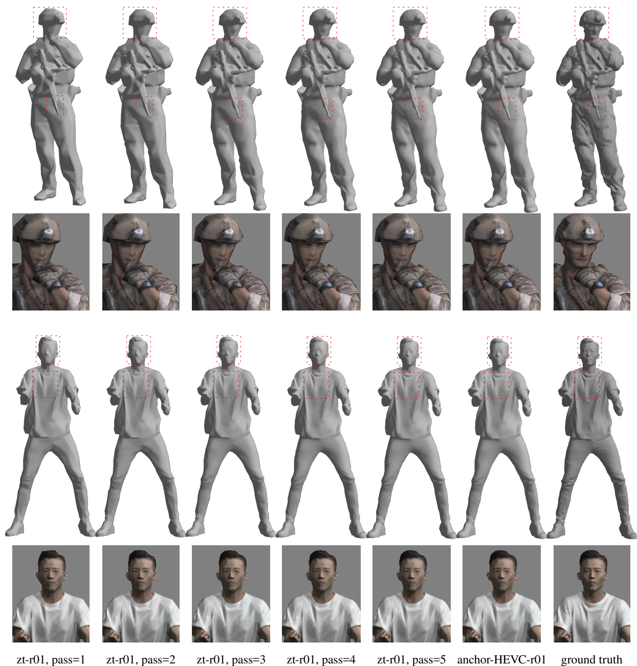
Figure 4.12: Examples of progressive geometry reconstructions from our zerotree method, using (left to right in each row): 1, 2, 3, 4, 5 zerotree passes corresponding to “zt-r01” from Figure 4.10, compared to the non-progressive reconstruction using HEVC-encoded displacements at the same CTC rate point (r01), and the ground truth (original input mesh) shown at the far right. The red rectangles outline regions where geometric changes are particularly noticeable. Corresponding reconstructions with near-lossless texture compression applied on top are shown underneath.
