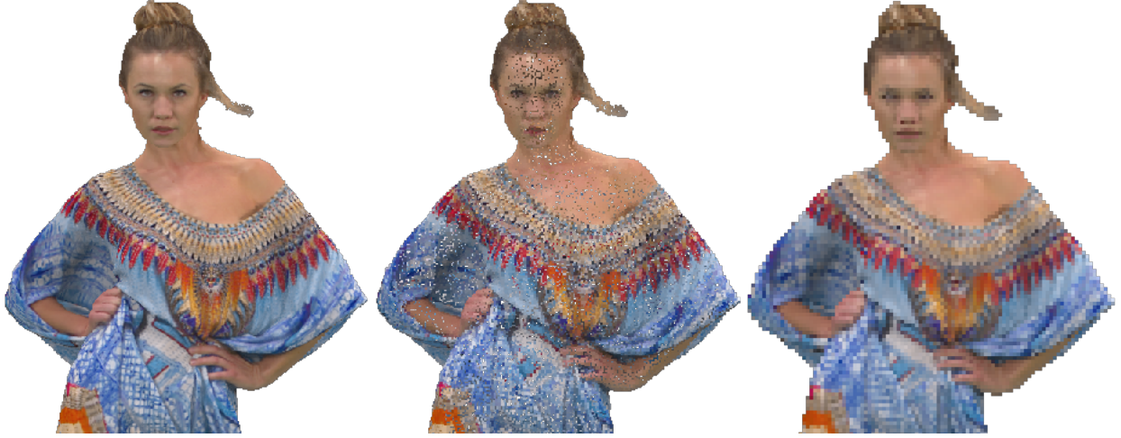
Figure 3.1: Comparison of downsampling approaches. Original point cloud (857,966 voxels), set downsampling (64,176 voxels D1_{\text{PSNR}} = 61.5\text{dB} ), and grid downsampling (62,130 voxels, D1_{\text{PSNR}} = 58.4\text{dB} ).
