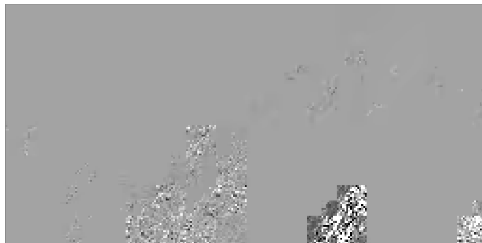
Figure 2.29: Packed wavelet coefficients of the displacements into a video frame. Gray regions represent zero-valued coefficients, while black and white represent positive and negative coefficients. The coefficients from each LoD are arranged in a block-aligned packing scheme, with ascending LoDs placed from left to right and bottom to top. Gray padding blocks are inserted both to maintain alignment with block boundaries and to fill the frame to its full size.
