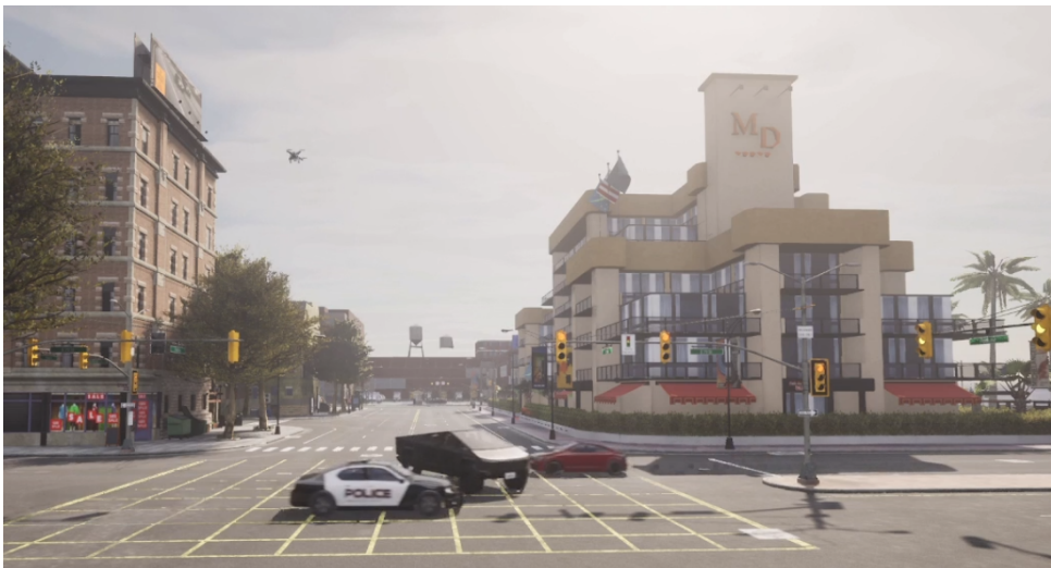
Figure 17 – A picture illustrating an attack in the Left Turn Assist scenario. The Tesla Cybertruck does a improperly timed left turn and ends up colliding with a police vehicle. The spoofer drone can be seen in the sky, close to the intersection.
