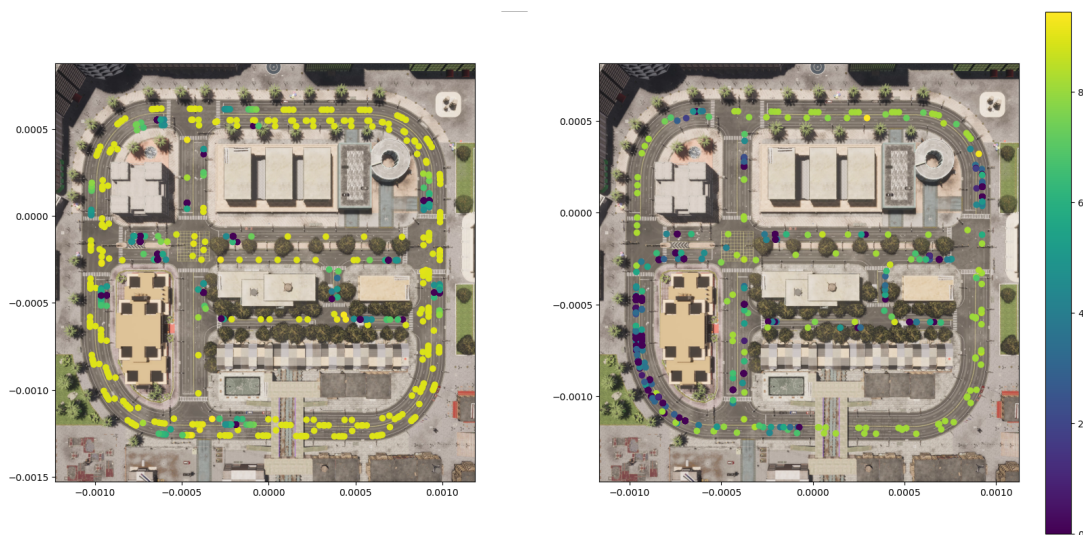
Figure 6 – Traffic comparison, on the left the light traffic simulation, and on the right the heavy one. Points represent the vehicle location and the speed during collection step. Right color map is represented in meters per second.
