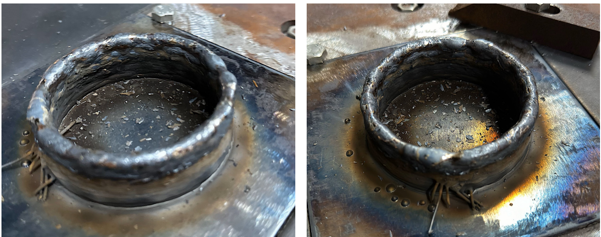
Figure 18 – Pictures taken from the deposited part of the first step-by-step successful experiment.
