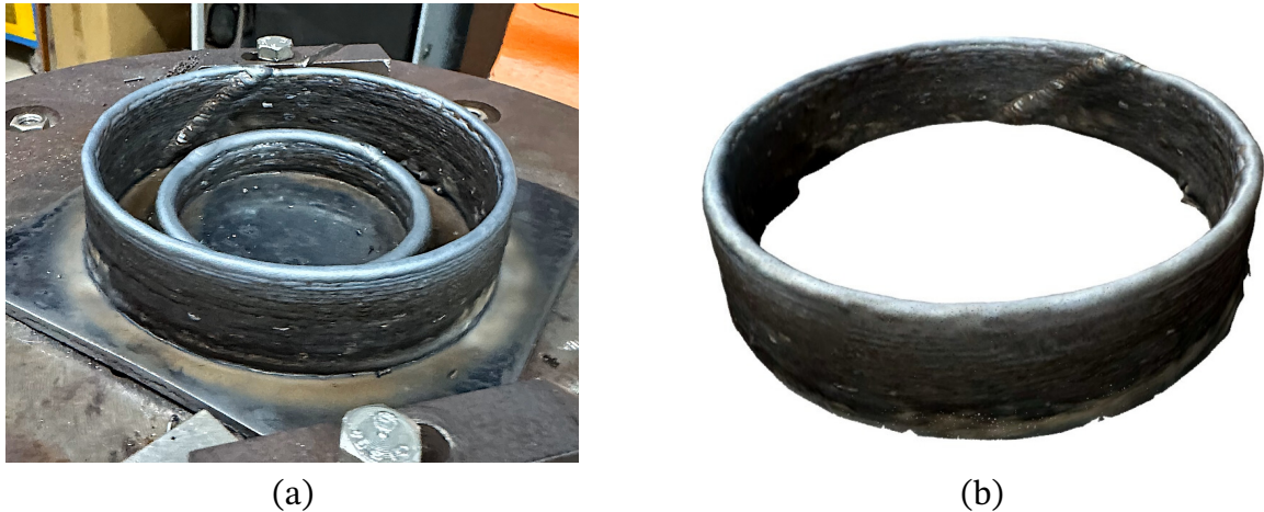
Figure 29 – (a) Real picture from the third experiment’s part (the outer tubular wall), (b) Scanned 3D model of the third experiment’s part.
