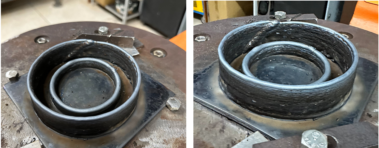
Figure 22 – Pictures taken from the deposited part resulting from the third successful experiment (the outer metal part, the inner one is the part from the second experiment).
