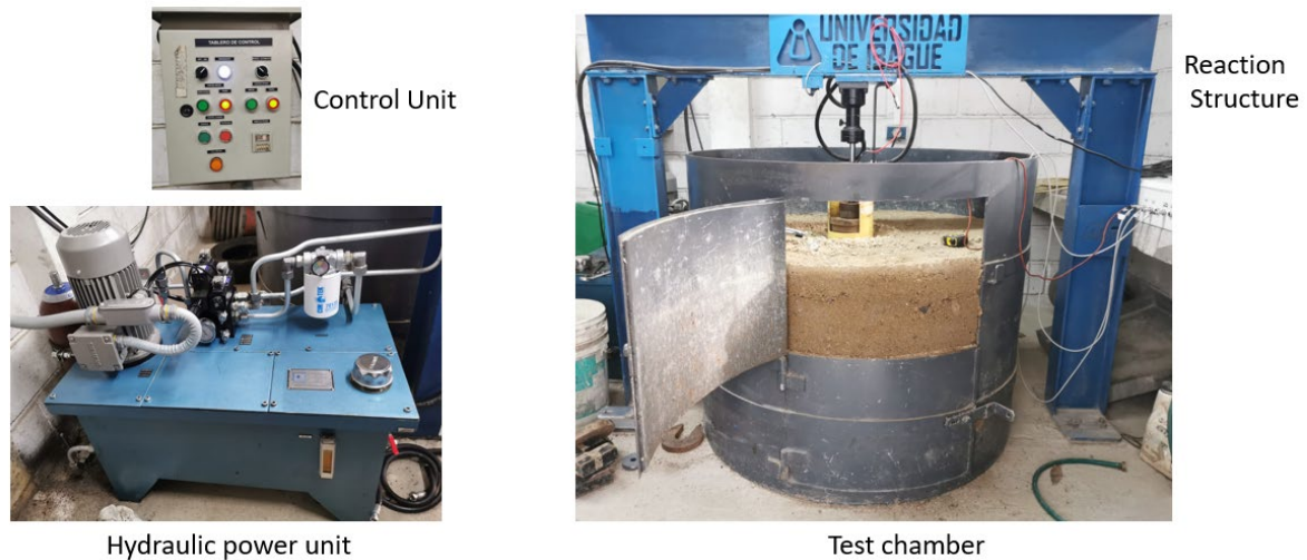
Figure 3.11 - Cyclic loading equipment used.
