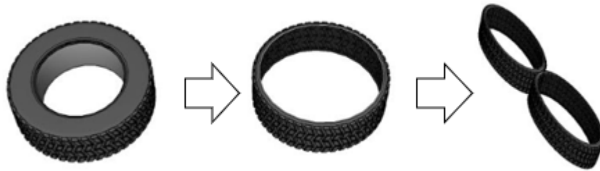
Figure 3.1- Design of the Process for Manufacturing Geocells with Used Tires.
