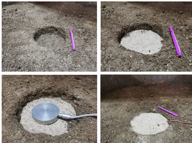
Figure 3.20 - Sequence of voltage cell installation.
