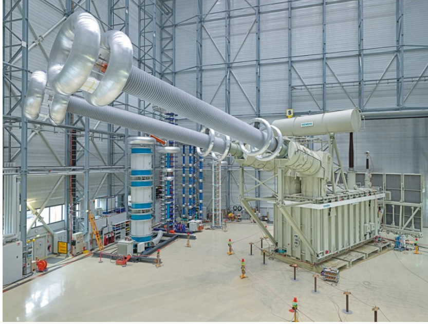
Figure 2.16: 1100 kV HVDC converter transformer by Siemens.
