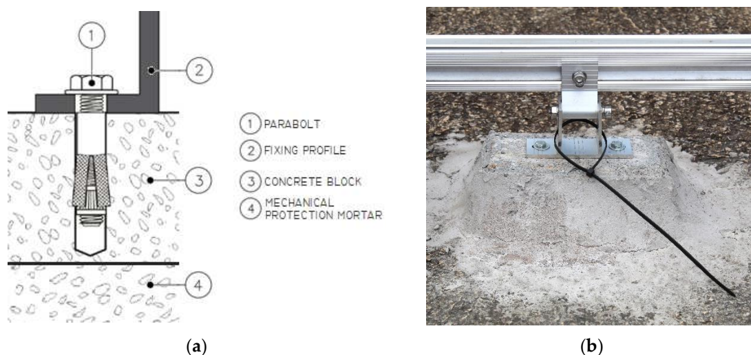
Figure 3. Fixing the photovoltaic panels to the roof: (a) construction detail; (b) execution photo. Source: the authors.
