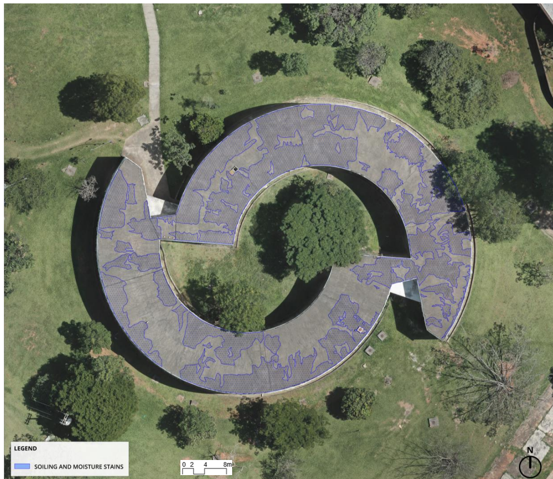
Figure 5. Damage map of the roof of the Sustainable Development Center: highlighting soiling and moisture stains. Source: the authors.
