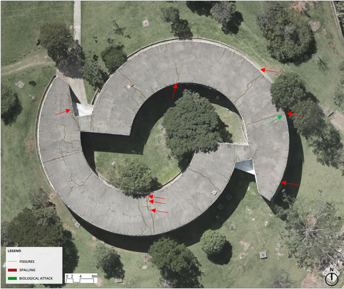
Figure 6. Damage map of the roof of the Sustainable Development Center: highlighting cracks, spallings, and stains from biological attacks. Source: the authors.
