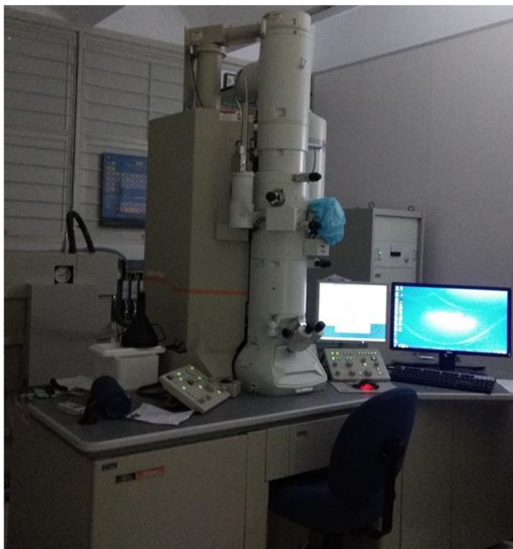
Figure 2. – Photograph of the JEM2100 electron microscope used for the experiments at LabMic. Photograph taken from [42]
