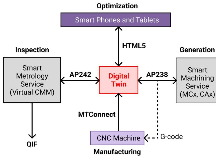
Figure 4.3: Digital Twin framework for machining proposed by STEP Tools, Inc. [54].
