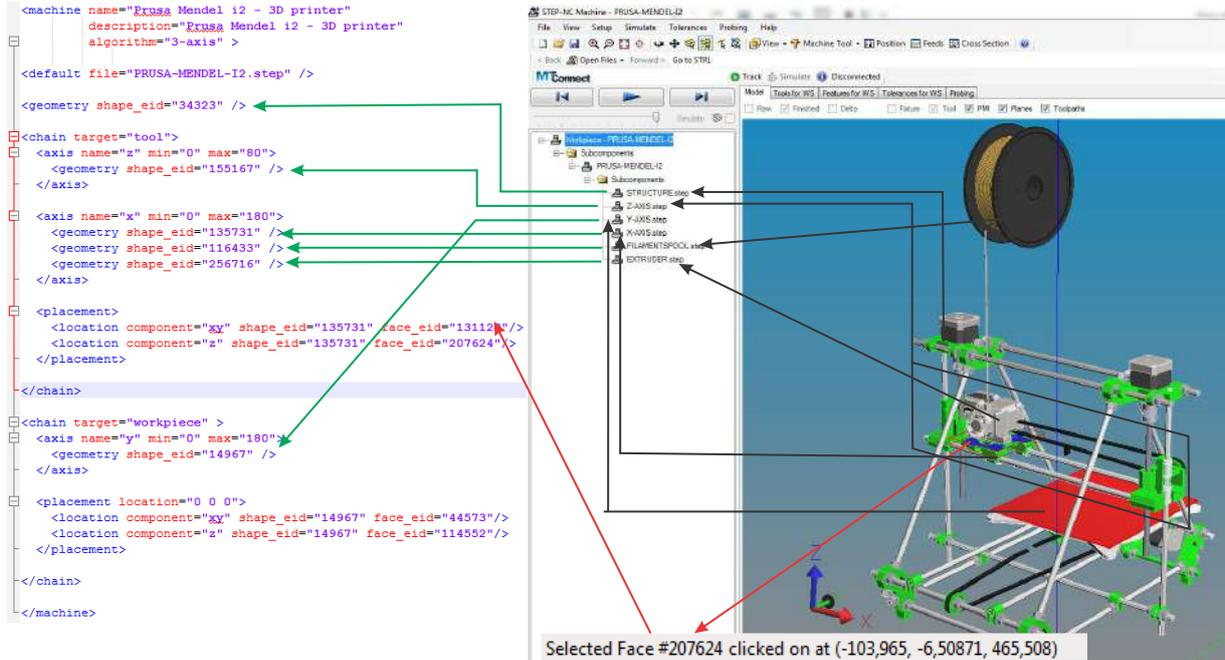
Figure 7.8: Configuring the 3D printer kinematic model into the STEP-NC Machine software.
