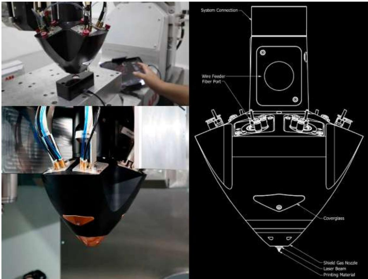
Figure 2.17: Meltio's wire-laser 3D print system for LDM
