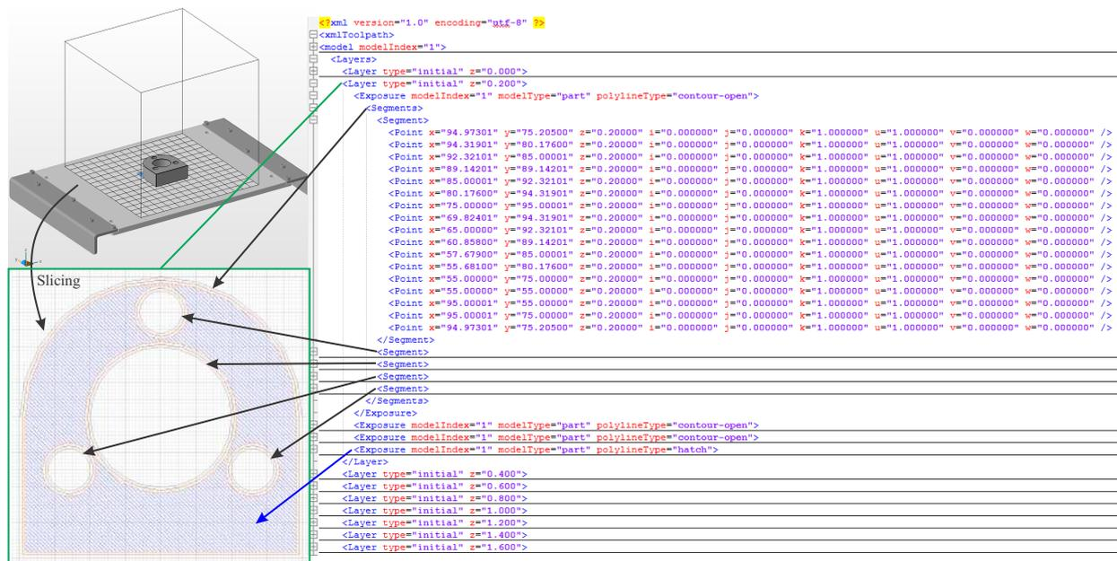
STEP-NC models, embedding machining data, and exporting files in either Part 21 or Part 28 formats. The adapter software parses the XML data by creating instances of classes specifically designed to represent the hierarchical structure of layers, exposures, segments, and points defined in the XML file. These instances are stored in memory and subsequently mapped to corresponding STEP-NC definitions.
