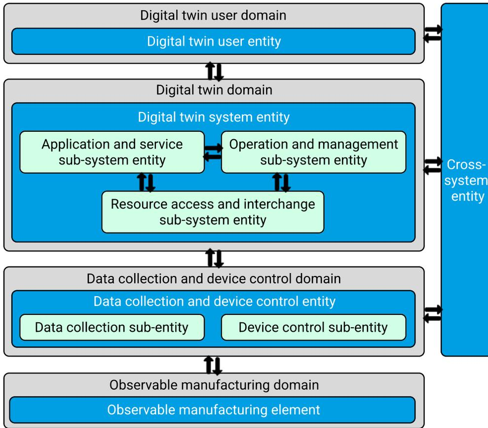
Figure 4.4: DTw framework for manufacturing from ISO 23247 Part 2 [232].
