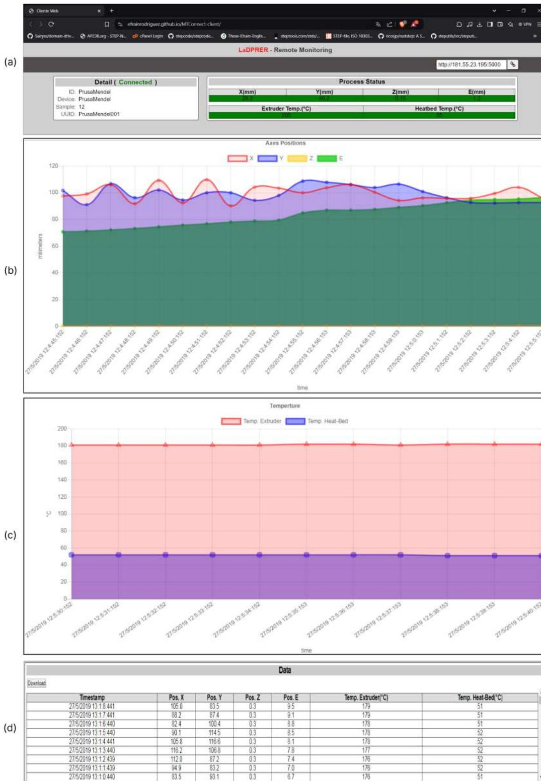
Figure 7.12: MTConnect web client for AM process monitoring.
