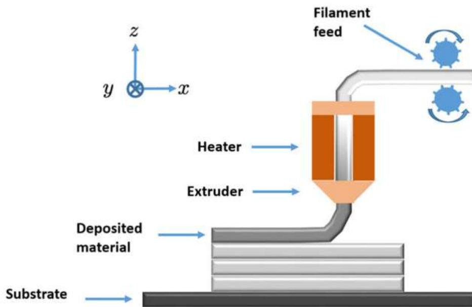
Figure 2.18: Material Extrusion (MEX) [169]
