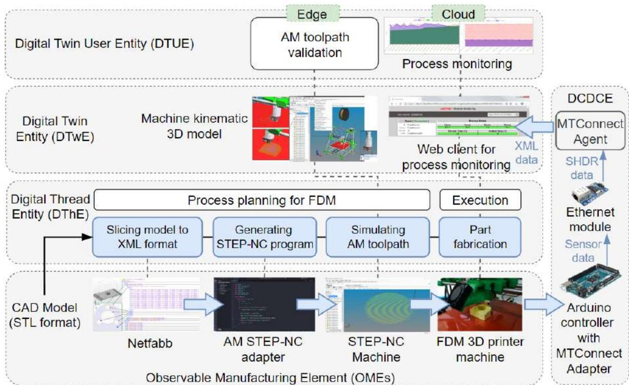
Figure 7.4: STEP-NC and MTConnect implementations in AM through digital ecosystem framework.
