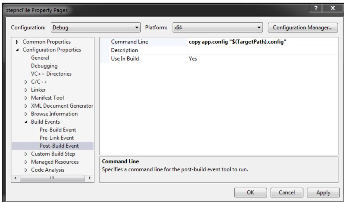
An important step is to add the **stepnc.dll** as within the reference from the project to use its functions in the building the STEP-NC data. You can add that stepnc.dll accessing by **Common Properties->References** and clicking on **Add New Reference**.
