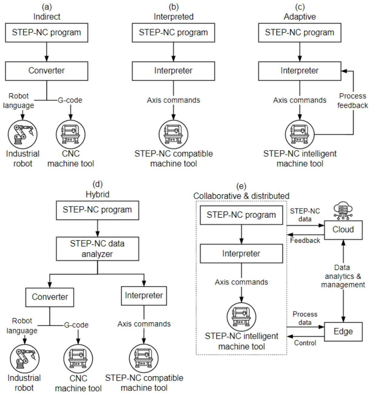
Figure 5.9: STEP-NC architectures in literature: a) Indirect; b) Interpreted; c) Adaptive; d) Hybrid; e) Collaborative.
