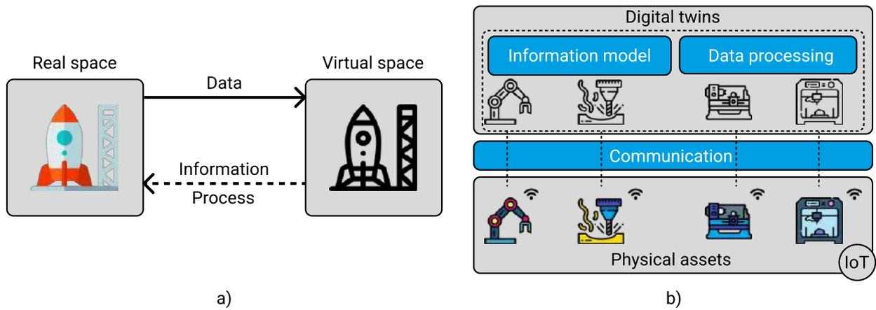
Figure 4.2: Three-dimensional reference models of Digital Twin: a) adapted from [216]; b) adapted from [37].
