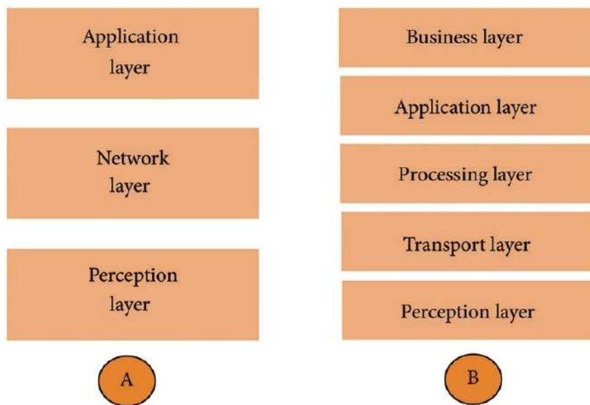
Figure 2.7: Fundamental IoT architectures: (A) Three layers; (B) Five layers. [122].
