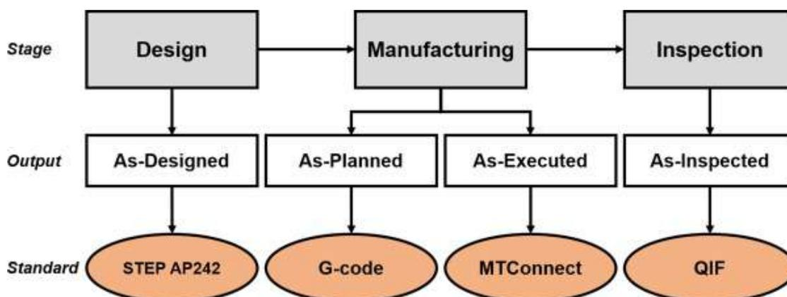
Figure 3.2: The vision of DTh from the NIST SMS Test Bed [189].
