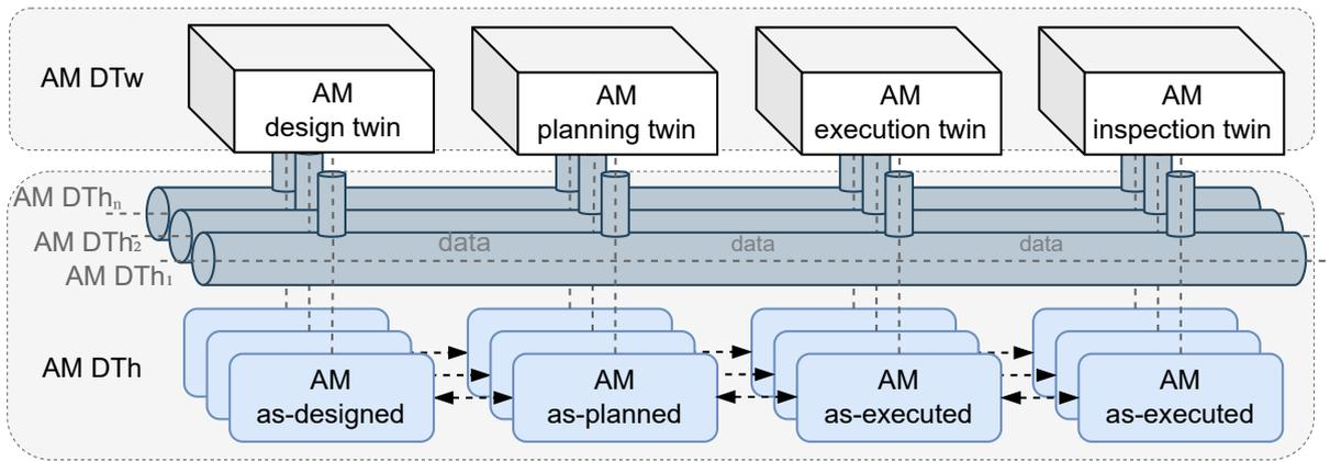
Figure 6.2: Concept of Multi-Threaded data flow interconnected with Digital Twins for cross-context lifecycle analysis.
