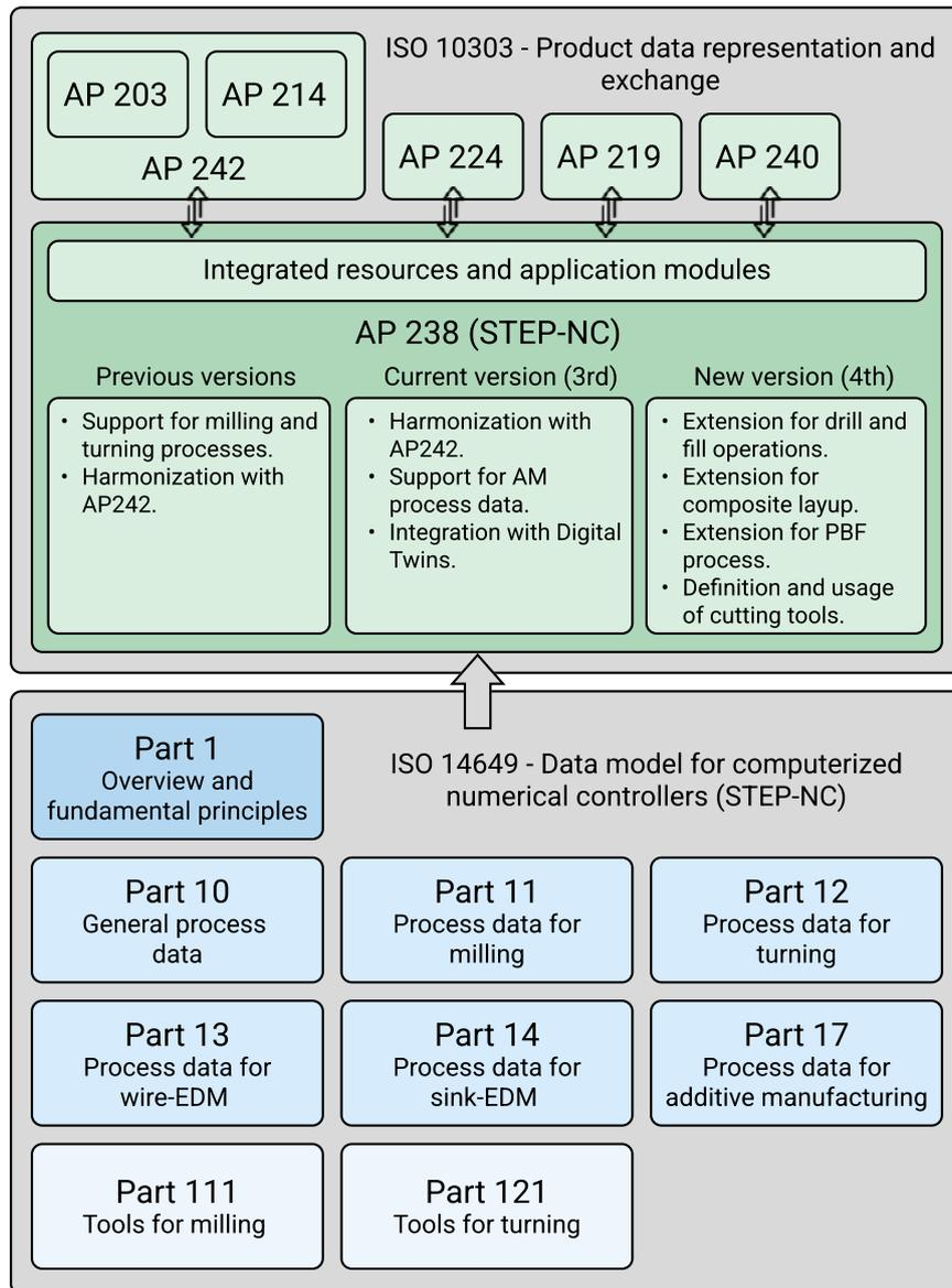
Figure 5.4: Overview of the structure of STEP-NC.
