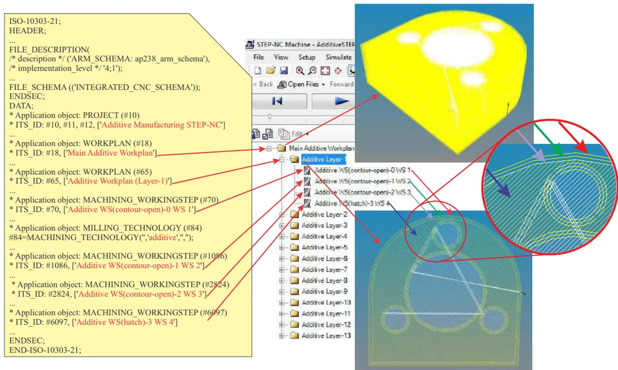
Figure 7.7: AM STEP-NC program and layers visualization in STEP-NC Machine software.
