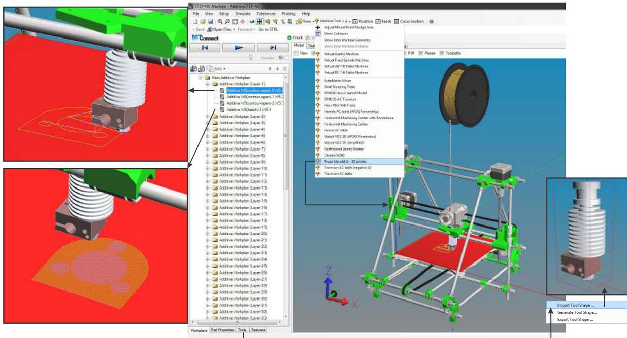
Figure 7.9: Simulation of the AM STEP-NC program with machine 3D model in the STEP-NC machine software.
