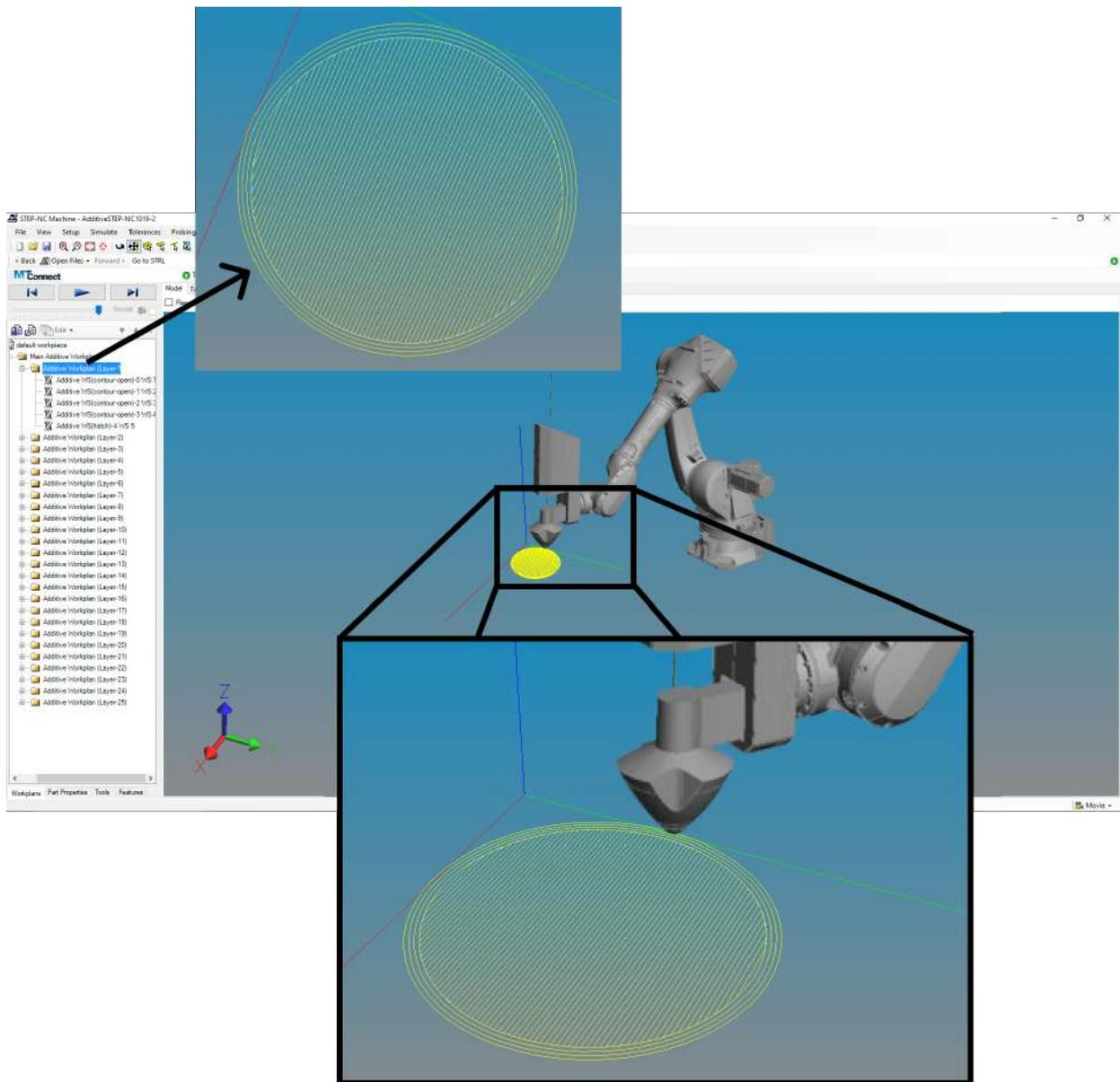
Figure 7.13: STEP-NC toolpath simulation for LMD process.
