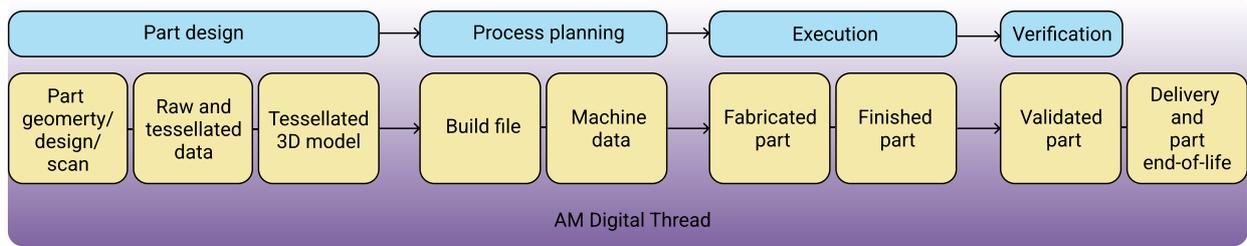
Figure 3.6: Overview of the AM Digital Thread. Adapted from [183, 186, 197]
