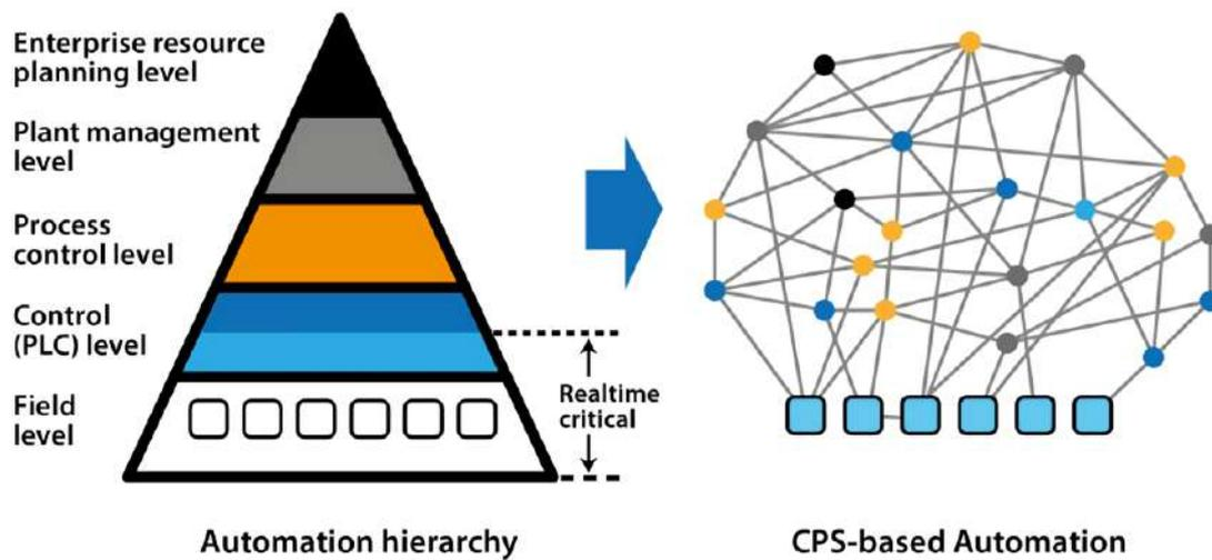
Figure 2.6: Decentralizing the traditional automation pyramid: A breakdown of the automation hierarchy through distributed services [34].
