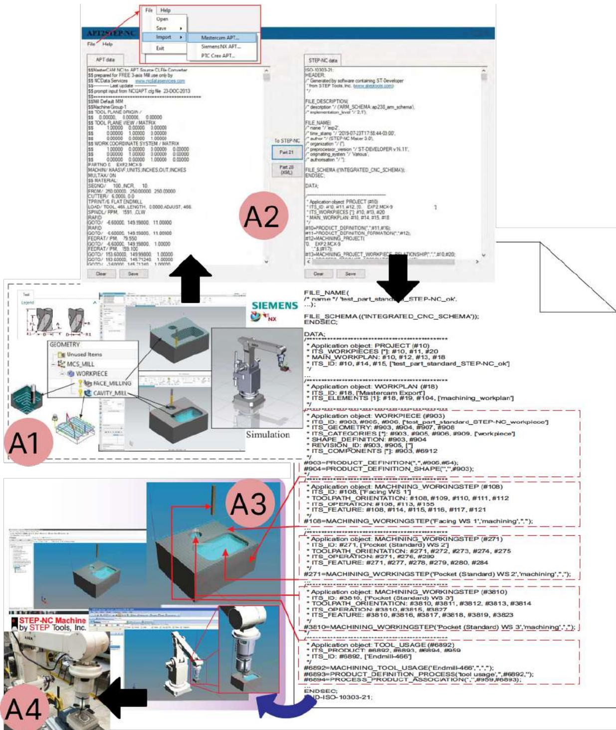
Figure 7.2: Workflow for generating a STEP-NC file from Mastercam machining data using an adapter.
