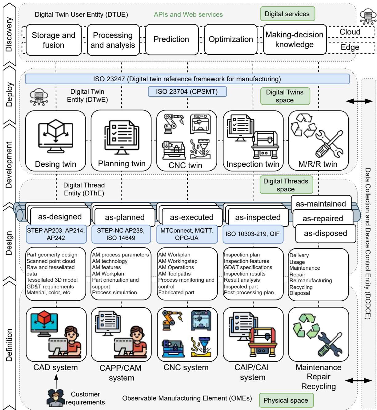
Figure 6.3: Digital ecosystem framework for AM driven by standards-based Digital Thread and Digital Twin.
