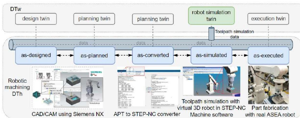
Figure 7.3: Overview of the robotic machining DTh.
