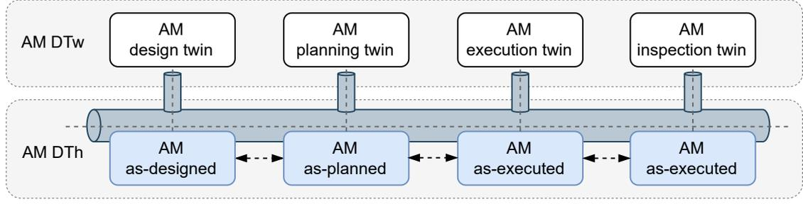
Figure 6.1: Concept of an AM Digital Thread connected with Digital Twins.
