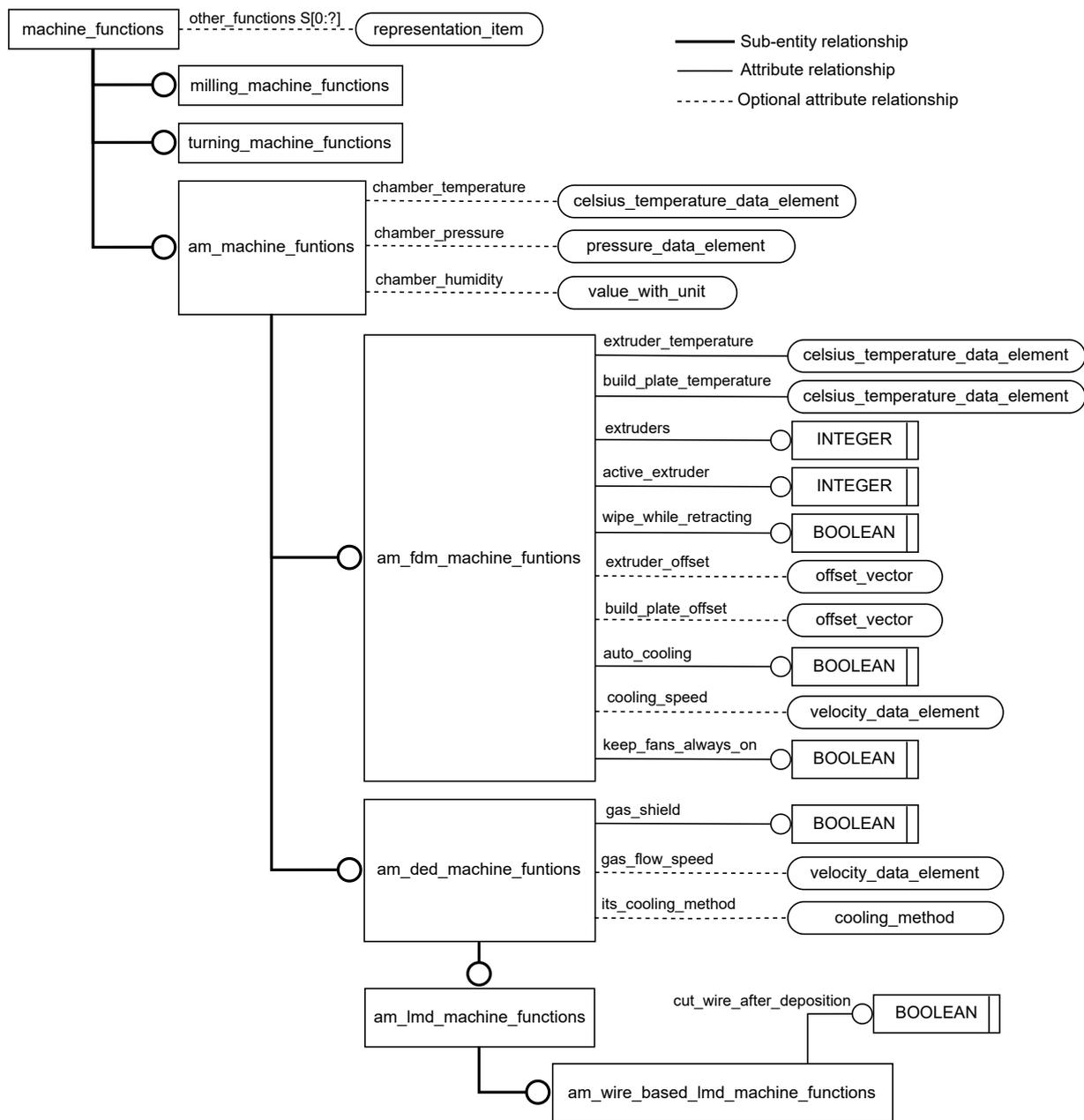
Figure 7.18: EXPRESS-G diagram of the proposed `am_machine_functions` entity.
