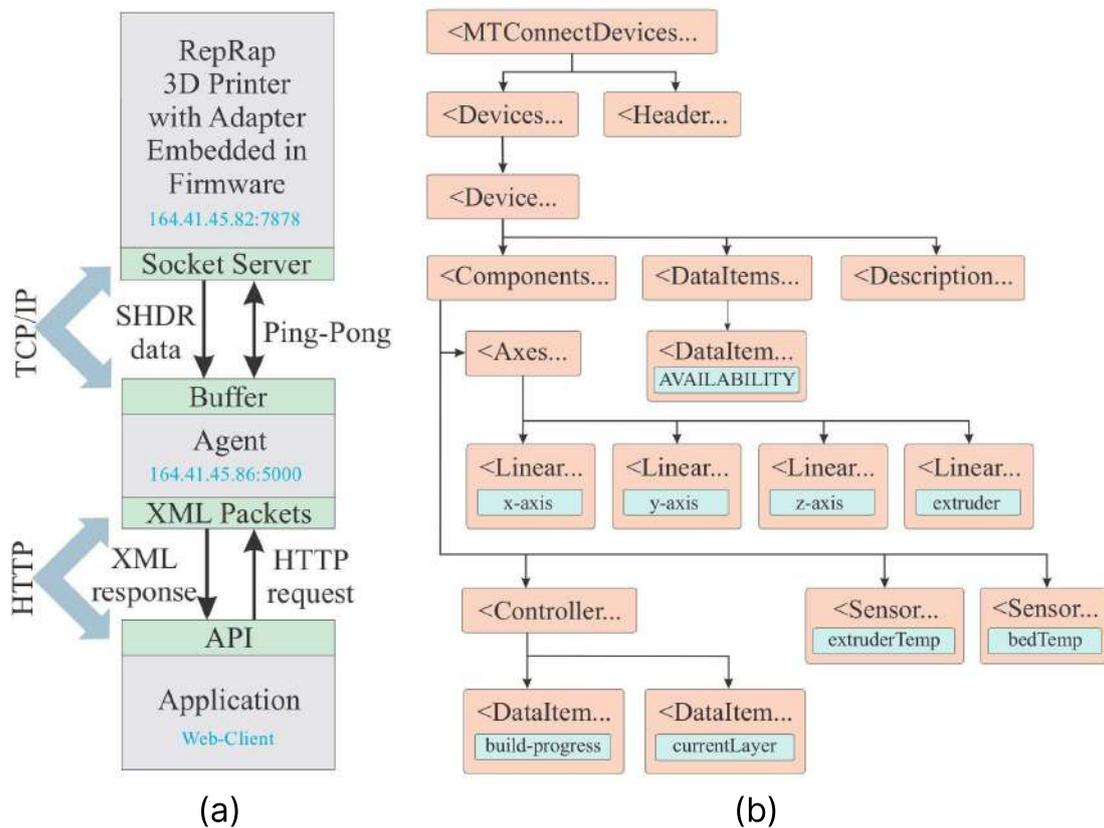
Figure 7.10: MTCConnect implementation: a) Architecture; b) 3D printer machine model.
