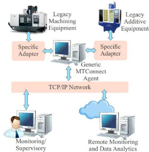
Figure 2.11: A typical data flow in MTConnect-based communication [146]
