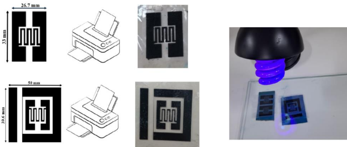
Figure 2.8 - Photomask Layout Showing Darkened Non-Circuit Areas and Transparent Circuit Traces
