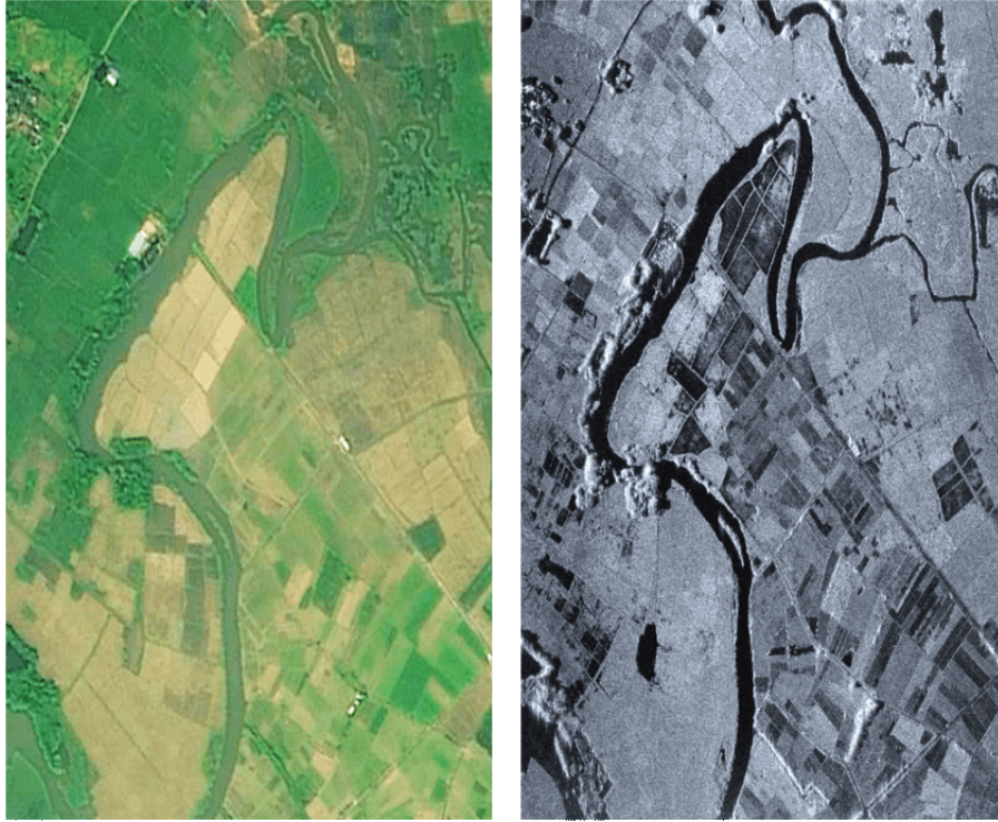
Figure 1.2. Comparison between a SAR image (on the right) and an optical image (on the left) of the same area. Source: Very-High-Resolution SAR Imaging with DGPS-Supported Airborne X-Band Data (ZHOU et al. , 2020)
