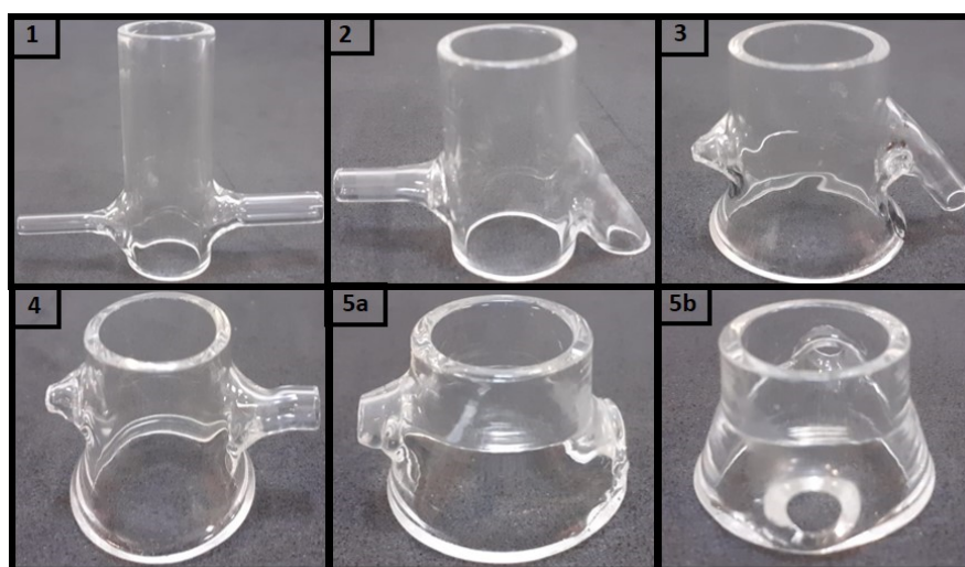
Figure 3. Images of the glass versions of the donor compartment: (1) first model without Db and angle \theta = 90^\circ ; (2) second model without Db and angle \theta < 90^\circ ; (3) third model with Db and angle \theta < 90^\circ ; (4) fourth model with Db and angle \theta = 90^\circ ; (5a) final model with Db and angle \theta < 90^\circ (side view), and (5b) final model with large output lacrimal flow (back view). The images are at different scales.
