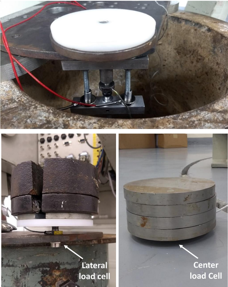
Figure 3.32. Assembly for the calibration of Futek load cells.
