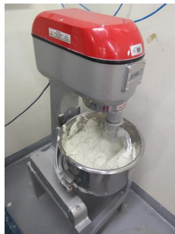
Figure 3.17. Mixing process of kaolin with water
