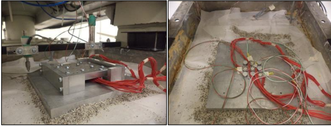
Figure 3.3. Assembly and instrumentation details of M3 model. (Rodríguez, 2016)
