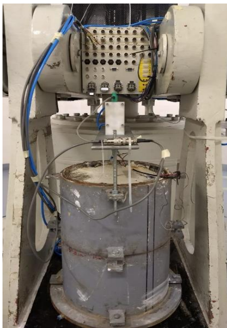
Figure 3.37. Container in the centrifuge platform.
