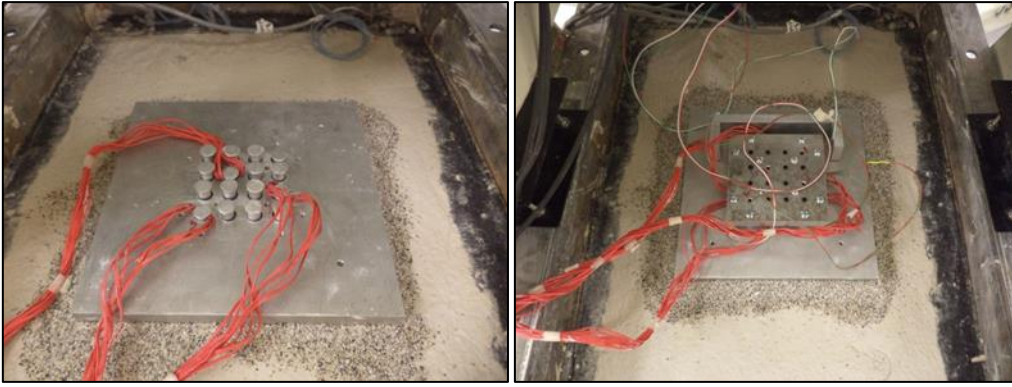
Figure 3.51. Assambly and instrumentation details of M4 model. Rodríguez 2016.
