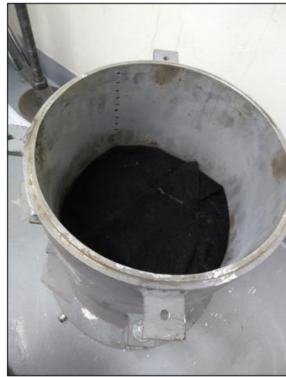
Figure 3.19. Mixture cover with geotextile
