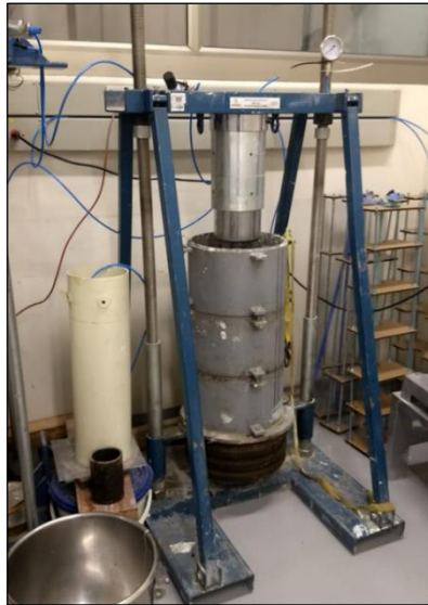
Figure 3.20. Loading with a hydraulic jack.
