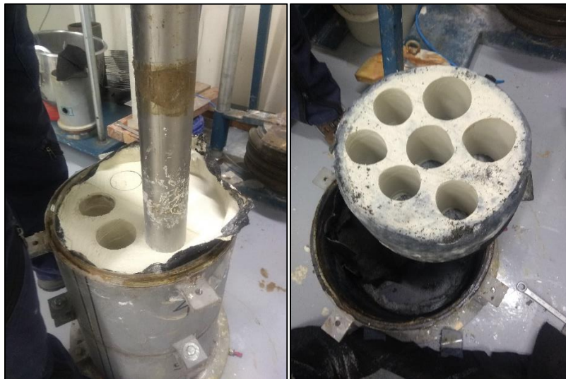
Figure 3.22. Container and extrusion of samples.
