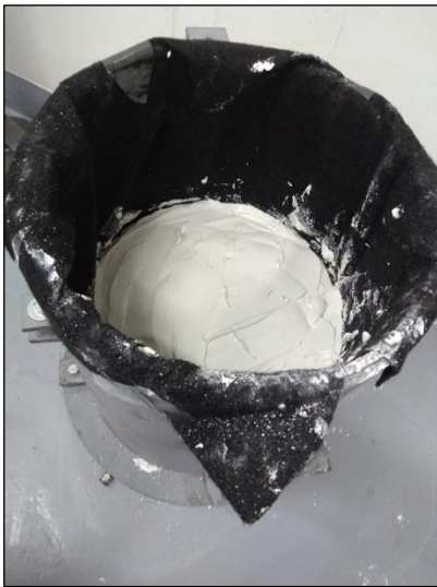
Figure 3.19. Mixture cover with geotextile
