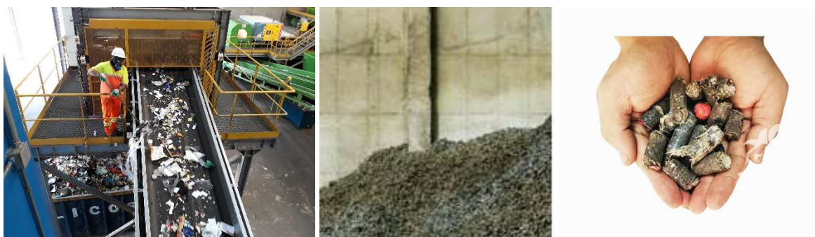
Figure 14 – From left to right: waste plant treatment in Brazil, picture from São Paulo City Hall. At the center, processed waste batch. At right, hand-size RDF fuel pellets.
