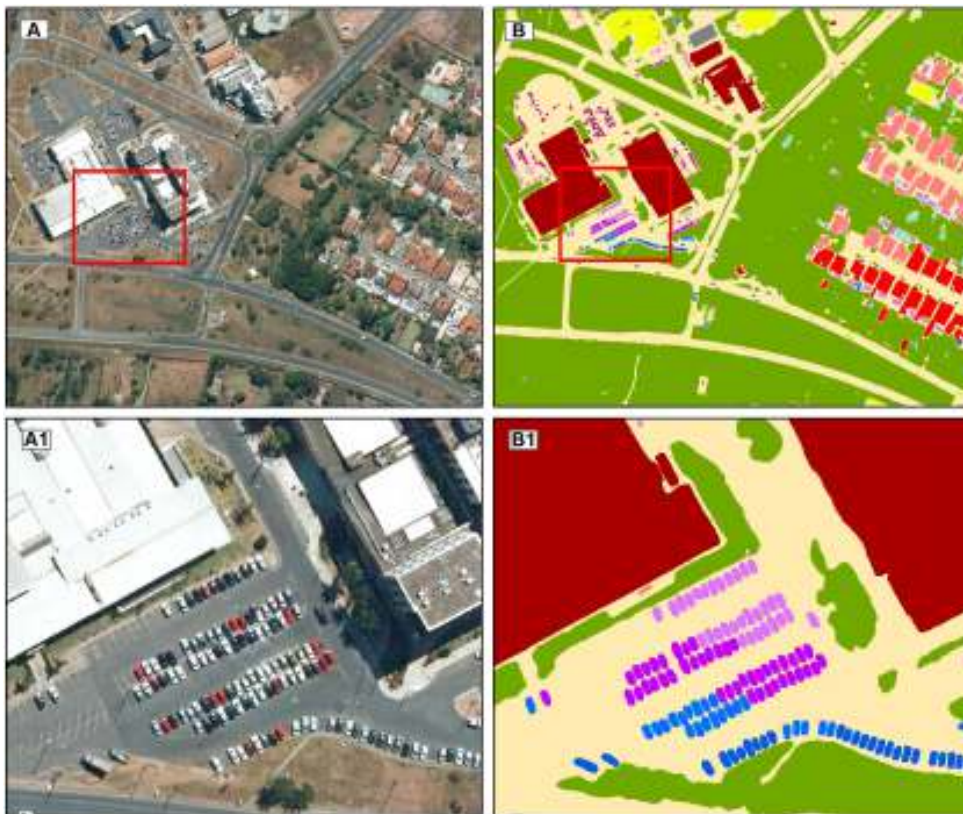
Figure (7.3) Original 2560x2560-pixel image (A) with its corresponding sliding windows panoptic results (A1) and a zoomed area from the image (A1) and prediction (B1).
