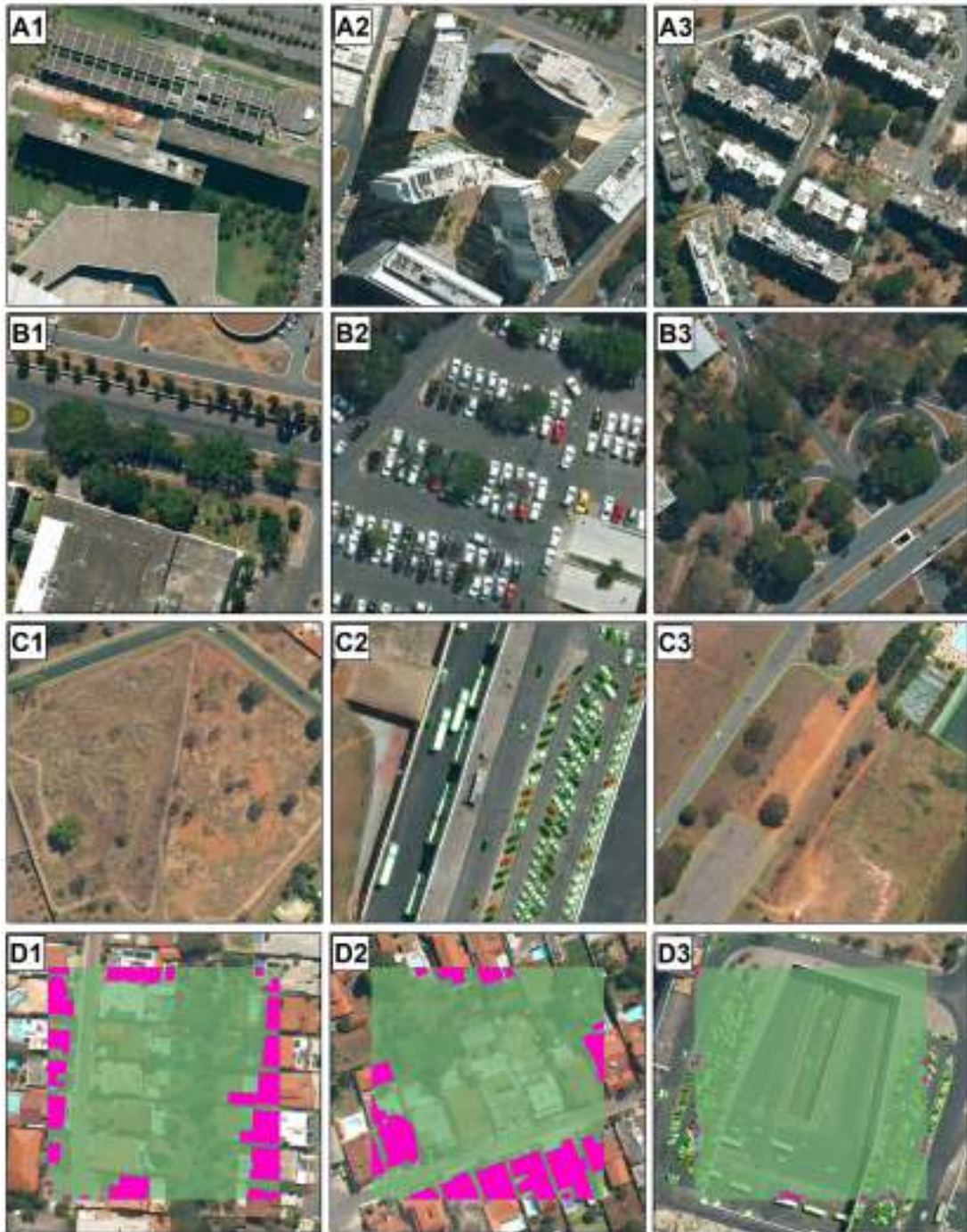
Figure (6.9) Three examples of (1) shadow areas (A1, A2, and A3), (2) occluded objects (B1, B2, B3), (3) class categorization (C1, C2, and C3), and (4) edge problem on the image tiles (D1, D2, and D3).
