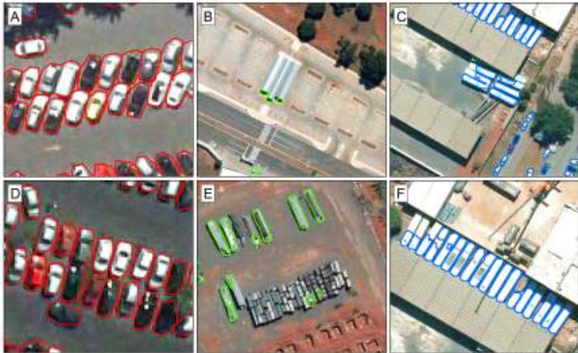
Figure (5.9) Errors in the classification procedure, and errors present from the conversion from polygon to raster.
