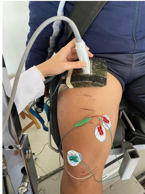
Figure 2 – A custom-made device to held the ultrasound probe for preventing it from moving.
