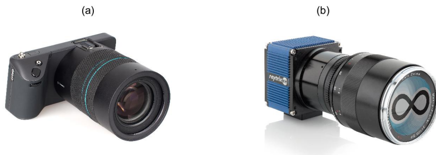
Figure 2.2.1: (a) A two-plane plenoptic to parameterize a 4D light field, and (b) Spatial multiplexed imaging system to acquire a 4D light field.
