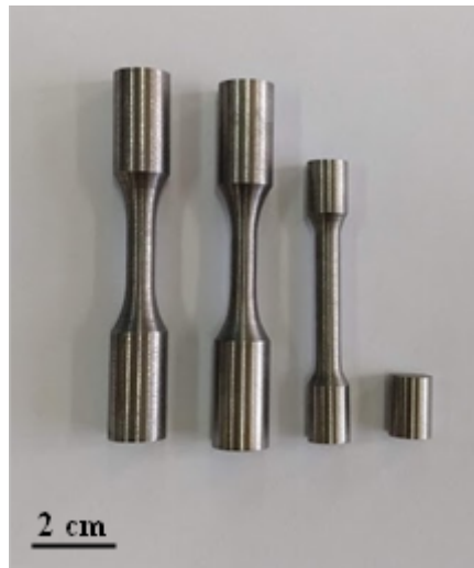
Figure 4.3. Manufactured specimens. From left to right: Bauschinger effect, tensile test and compression test.
