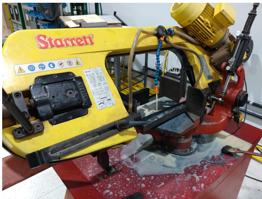
Figure 4.7. Starrett S3720 bandsaw during cutting procedure.
