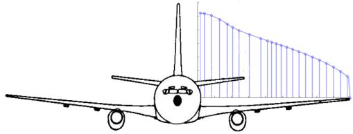
Figure 20: Example of shear force distribution along semispan of jet transport aircraft ((M∞ = 0.80, C<sub>L</sub>=0.48, *n*=1)
