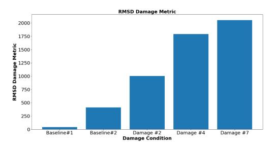
Figure 25: Specimen #1 and some RMSD damage metrics.
