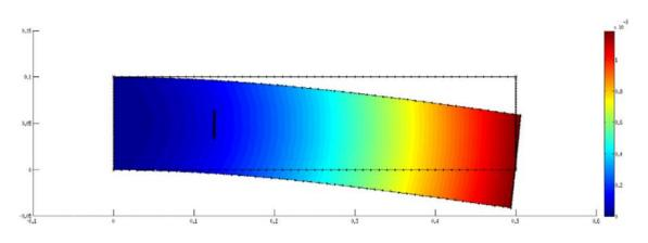
Figure 27 – Deformed shape of cantilever beam case with noise.
