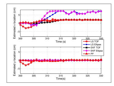
Figure 44: Least squares, extended Kalman filter, and particle filter convergence for both oneway ultrasonic pulse measurement models with the heating source located at (x = 2cm, y = 0cm)and an initial guess of (x = 0cm, y = 0cm).
