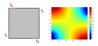
Figure 12: initial domain (left) and the initial temperature map (right)
