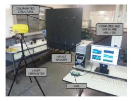
Figure 22: Schematic of the experimental setup.
