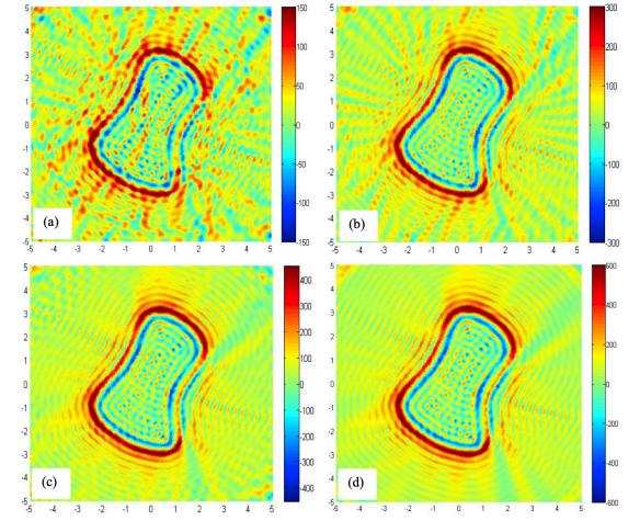
Figure 5: Identification of a single obstacle in an empty domain. Contour plots of  $D_T$  in terms of the number of sources: (a) N = 25, (b) N = 50, (c) N = 75 and (d) N = 100.
