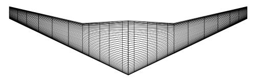
Figure 40: TRE-planform with surface mesh
