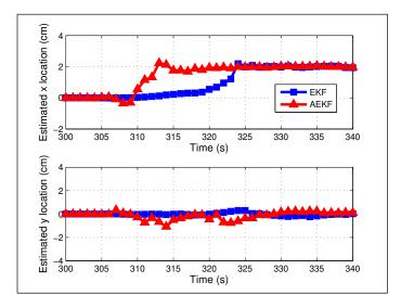
Figure 54: Extended Kalman filter and adaptive extended Kalman filter convergence with  $Q_0 = 1-4m^2 \times I_2$ ,  $R = 4-7 \times I_4$ , and M = 2. The heating source is located at (x = 2cm, y = 0cm) with an initial guess of (x = 0cm, y = 0cm).
