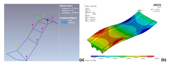
Figure 17 – Third frequency mode shapes of intact beam: (a) experimental (27.29Hz), (b) numerical (25.72Hz).
