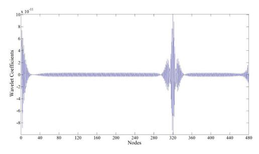
Figure 25 – Wavelet coefficients DWT using bior3.7 for cantilever beam case.
