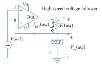
Figure 9: Electronic circuit used to measure  $i(\omega, t)$ . Source Maruo *et al* (2015).
