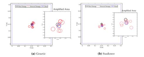
Figure 28: Structural damage (holes) detection in composite plate using GA and SFO algorithm.
