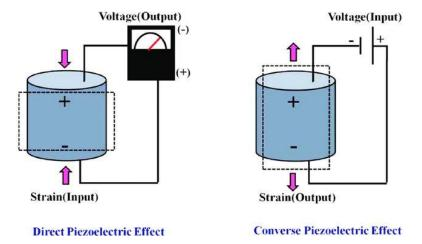
Figure 3: Direct and inverse piezoelectric effects. Source: Lakshmi et al, 2018.
