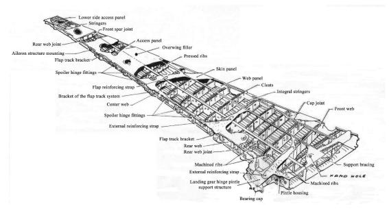
Figure 14: Illustration of a wingbox of a cantilever wing (Drawing from ITA's Aircraft Design Department)
