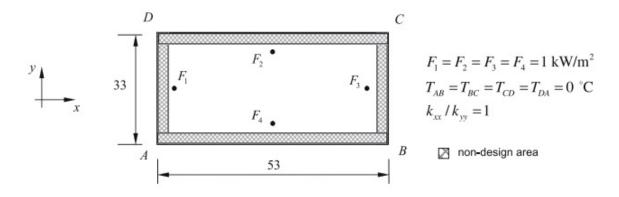
Figure 6: Initial design for the PCB
