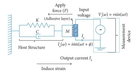
Figure 4: Mechatronic 1 DOF model of the coupled electromechanical transducer (source Maruo *et al* (2015)).
