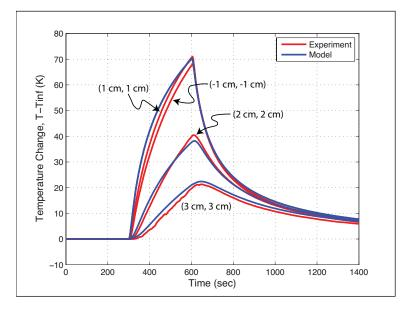
Figure 22: Comparison of the temperature response on non-heated side of the plate at four sensor locations.
