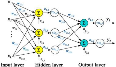
Figure 57: Exemplification of a multi-layer feed-forward network
