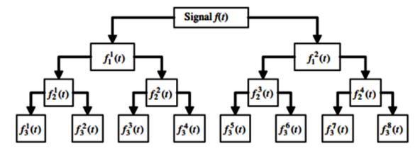
Figure 18- Wavelet Packet Decomposition (WPD) (adapted from Peng, Hao and Li, 2012).
