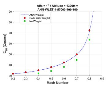
Figure 66: Induced drag coefficient for airplane 156218 at  $\alpha$ =1° at an altitude of 13,000 m
