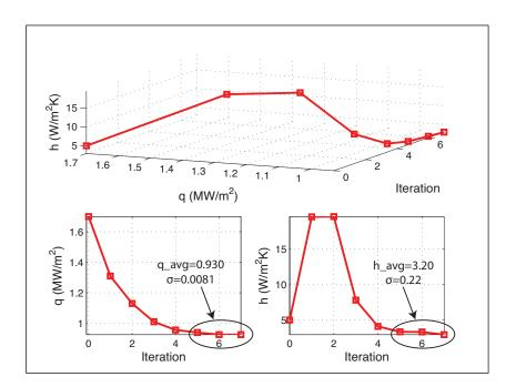
Figure 20: Extended Kalman filter and extended information filter convergence. The filters produce identical results and are presented together.
