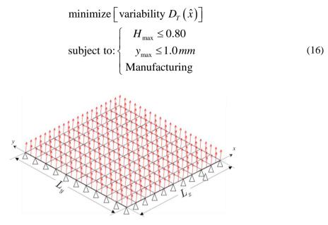
Figure 46: Square plate simply supported on the edges, with uniformly distributed loading along the entire surface, represented in a simplified way by the vectors in red.
