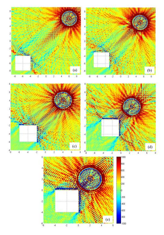
Figure 11: Identification of the square obstacle in the presence of a preexistent circular obstacle. Contour plots for the topological derivative results as function of the distance between obstables: (a)  $d/r = 6\sqrt{2}$ , (b)  $d/r = 5\sqrt{2}$ , (c)  $d/r = 4\sqrt{2}$ , (d)  $d/r = 2.5\sqrt{2}$ , (e)  $d/r = 2\sqrt{2}$ . The same color scale is used in all subfigures.
