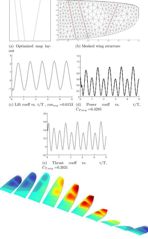
(f) Deformation of wing over a flapping cycle
