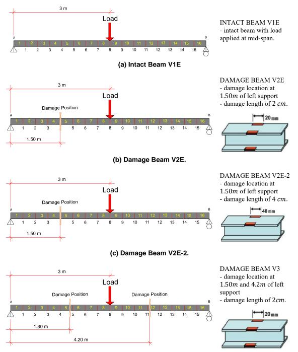
Figure 2 – Schematic description of induced damage for each experimental static essays
