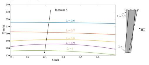
Figure 82: Influence of taper ratio on the flutter speed
