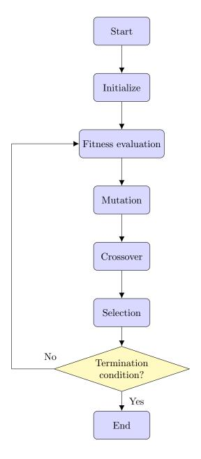
Figure 7: Schematic representation of the DE workflow.
