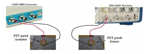
Figure 7: Graphic representation of the process of connections between PZT inserts and acquisition system equipment.
