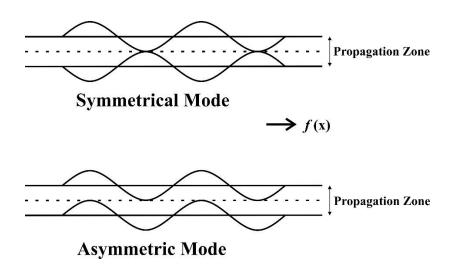
Figure 4: Symmetric and anti-symmetric patterns.
