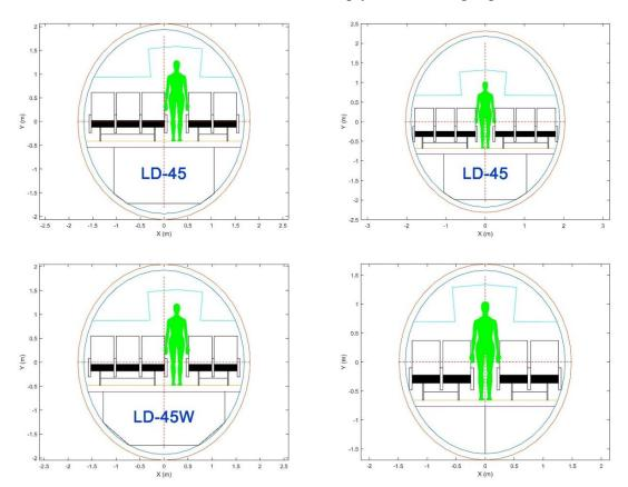
Figure 78: Examples of fuselage cross-sections
