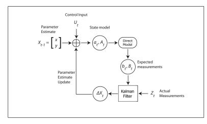
Figure 5: Parameter estimate update process using the Kalman filter and a direct model.
