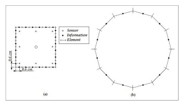
Figure 62: Elastostatic model: (a) discretization of the plate and positioning of sensors, (b) discretization of the hole.
