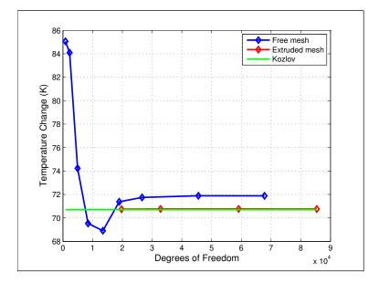
Figure 16: Grid independence results for the heated side at 1.4cm from the source and t = 400s.
