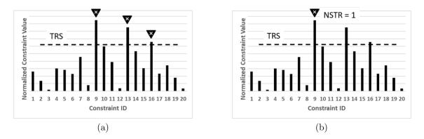
Figure 3: Schematic illustration of the combined constraint freezing/constraint freezing procedure. Constraints are normalized.
