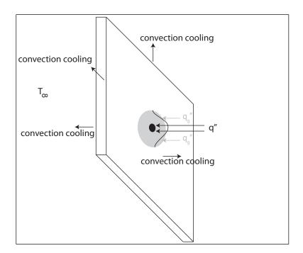
Figure 18: Illustration of boundary conditions on the flat plate.
