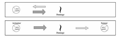
Figure 1: Pulse-echo and pitch-catch approaches in Lamb Waves techniques.
