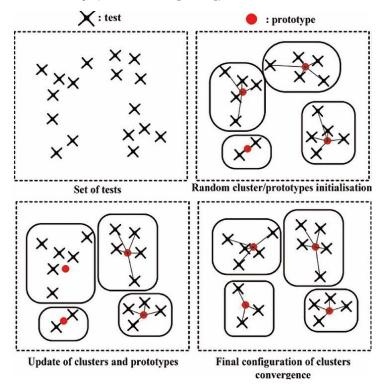
Figure 3 – Scheme representing the dynamic clouds algorithm.
