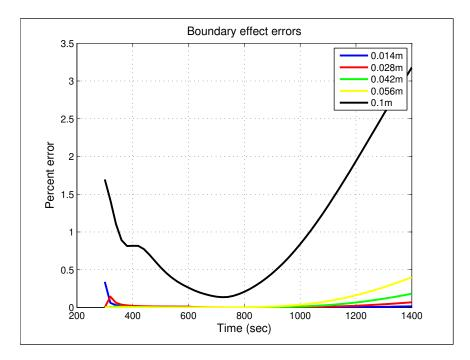
Figure 24: Illustration of when and where the plate edges introduce errors in the temperature distribution.
