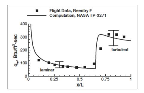
Figure 2: Heating profile on a ballistic RV, peak Mach=20 Schneider [2004].
