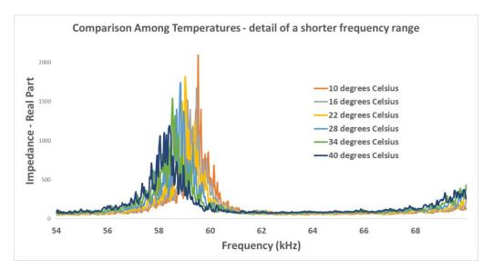
Figure 23: Specimen #1 and temperature changes for Baseline #1- shorter frequency range.
