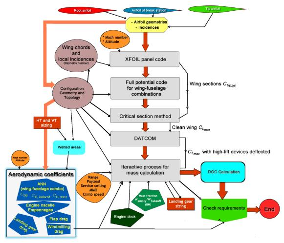
Figure 75: Workflow of the airplane analysis tool
