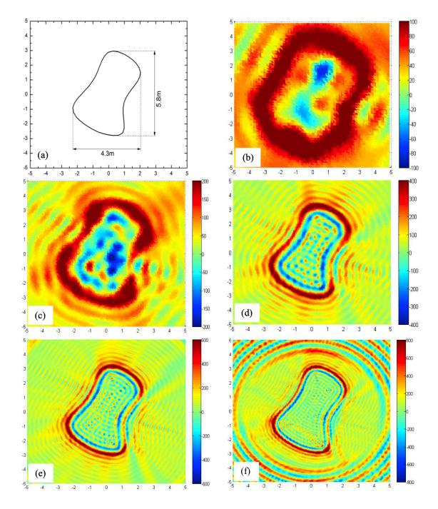
Figure 4: Identification of a single obstacle in an empty domain. Contour plots of  $D_T$  for different illumination wavelengths: (a) Geometry of the hidden obstacle and results for the obstacle shape for (b)  $\lambda/D = 0.85$ , (c)  $\lambda/D = 0.425$ , (d)  $\lambda/D = 0.213$ , (e) $\lambda/D = 0.142$  and (f)  $\lambda/D = 0.106$ .
