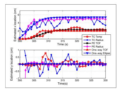
Figure 30: Extended Kalman filter convergence for all six measurement models with source at (6cm, 0cm) and initial guess of (0cm, 0cm).
