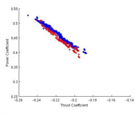
Figure 24: Collection of final Pareto fronts from 10 runs: fractone mapping in red, original mapping in blue
