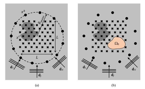
Figure 3: Topological derivative computation: (a) empty domain, (b) domain with a pre-existent obstacle. Symbols  $\bullet$  and  $\times$  indicate the positions of the receptors and the domain points, respectively.
