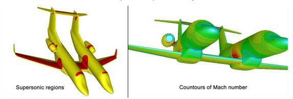
Figure 10: Euler calculation for a double-fuselage configuration (Mach = 0.76,  $\alpha$  = 0°). At left: red regions indicate supersonic flow. At right: red color and yellow colors are associated with lower speeds; green color indicates that the local speed is close to the freestream Mach number
