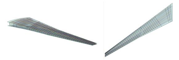
Figure 29: Structural layout of the rebuilt KC-135 wingbox
