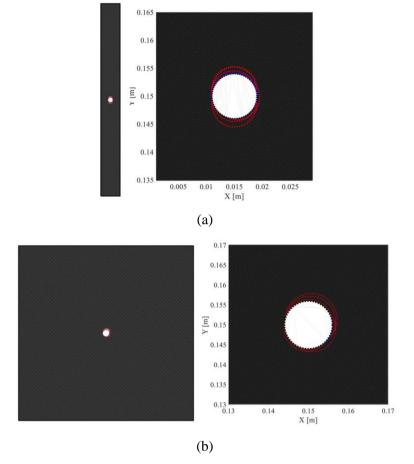
Figure 31: Experimental damage identification results considering: (a) the composite beam and (b) the composite plate.
