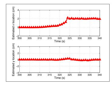
Figure 50: Extended Kalman filter convergence with the state model covariance values of  $Q = 1-4m^2 \times I_2$ , measurement covariance values of  $R = 4-7 \times I_4$ , heating source located at (x = 2cm, y = 0cm), and an initial guess of (x = 0cm, y = 0cm).
