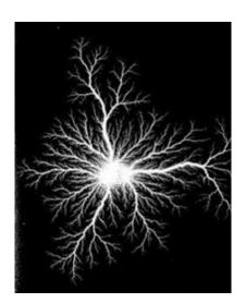
Figure 9: FL in tetra-fluoride gas under 30kV voltage and 30.3atm pressure (Pereira et al. [2021]).
