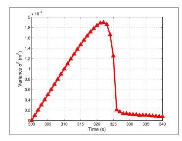
Figure 52: Variance  $(\sigma^2)$  from the state covariance matrix  $(\Sigma)$  for state model covariance of  $Q = 1-4m^2 \times I_2$  and measurement covariance of  $R = 4-7 \times I_4$ . The heating source is located at (x = 2cm, y = 0cm) with an initial guess of (x = 0cm, y = 0cm). Convergence (from Figure 50) is at 324s.
