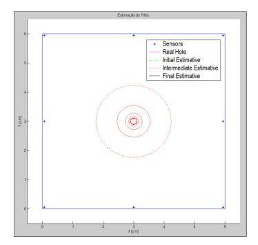
Figure 67: Performance of Kalman filter for a hole (3.00;2.00;0.06) cm for a potential model.
