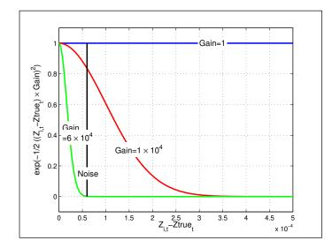
Figure 42: Comparison of selected particle filter gain values with sensor noise.
