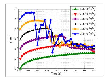
Figure 53: Variance  $(\sigma^2)$  from the state covariance matrix  $(\Sigma)$  for a range of state model covariance values (Q) and constant measurement covariance of  $R = 4-7 \times I_4$ . The heating source is located at (x = 2cm, y = 0cm) with an initial guess of (x = 0cm, y = 0cm). Convergence behavior can be found in Figure 47.
