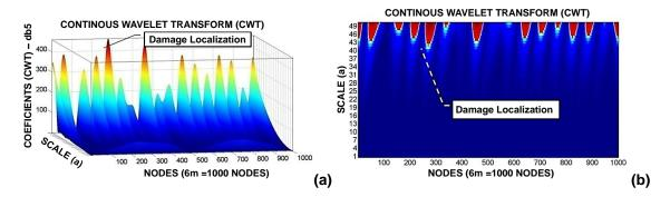
Figure 9 – CWT coefficients for beam V2E using db5: (a) 3D view and (b) 2D plan.
