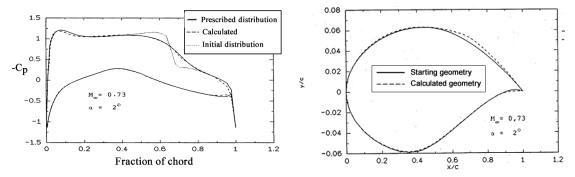
Figure 39: Example of the inverse technique application for airfoil design at a transonic condition ( $M_{\infty}$ = 0.73,  $\alpha$ =2°) [45] [47]
