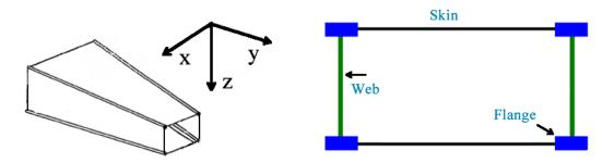
Figure 15: Simplified model of a wingbox
