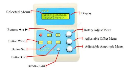
Figure 8: Function Generator - UDB11008S model.
