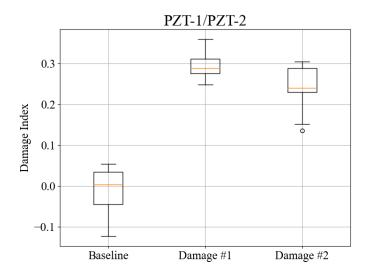
Figure 15: Boxplot of DI metric values for inspection path PZT-1/PZT-2.
