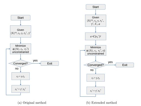
Figure 15: Interior penalty method for constrained optimization.
