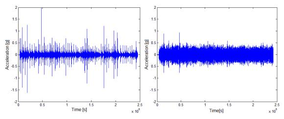
Figure 5: Example of vibration tests performed in laboratory: impact (left) and random (right).
