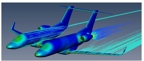
Figure 11: Streamlines over the dual-fuselage configuration (Mach = 0.76,  $\alpha$  = 0°). Surface geometry is colored according to the calculated Mach number. Notice the rapid expansion of engine exhaust gases
