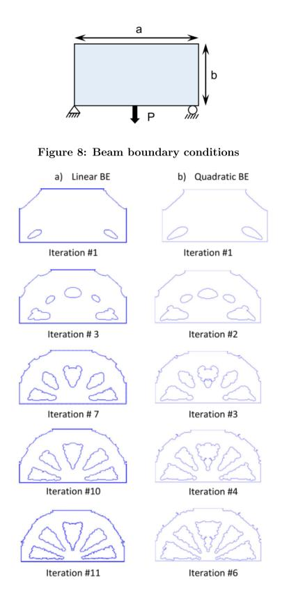
Figure 9: Beam topology evolution: a) linear and b) quadratic boundary elements
