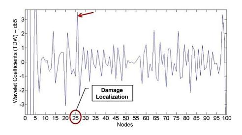
Figure 6 – DWT coefficients for V2E beam using db5.
