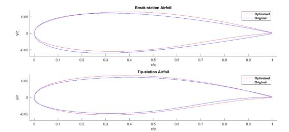
Figure 71: Break- and tip-station airfoils of the selected airplane optimal configuration
