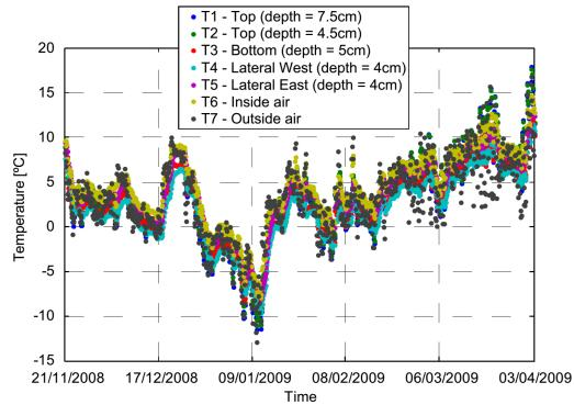
Figure 12. Time history of temperatures (before strengthening).
