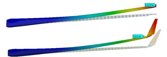
Figure 33: Calculated wingtip displacement in meters (Mach = 0.70,  $\alpha$  = 3.5°)
