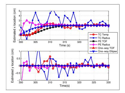
Figure 28: Extended Kalman filter convergence for all six measurement models with source at (2cm, 0cm) and initial guess of (0cm, 0cm).
