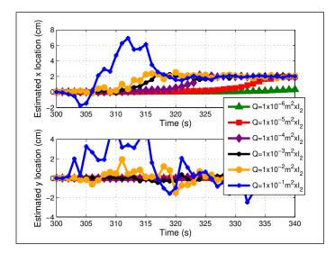
Figure 47: Extended Kalman filter convergence for a range of state model covariance values (Q) with constant measurement covariance values of  $R = 4-7 \times I_4$ , the heating source located at (x = 2cm, y = 0cm), and an initial guess of (x = 0cm, y = 0cm).
