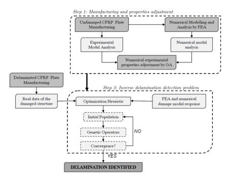
Figure 20: Flowchart of the delamination identification.
