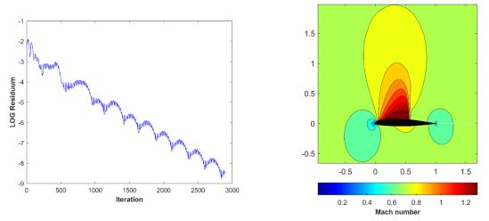
Figure 37: Solution of a transonic flow calculated over the airfoil ITADX4 with a full potential code ( $M_{\infty}$ = 0.73 and 1.5° angle of attack)
