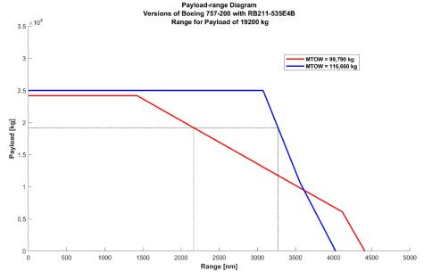
Figure 79: Payload-range diagram for some sub-versions of B757-200 [123]
