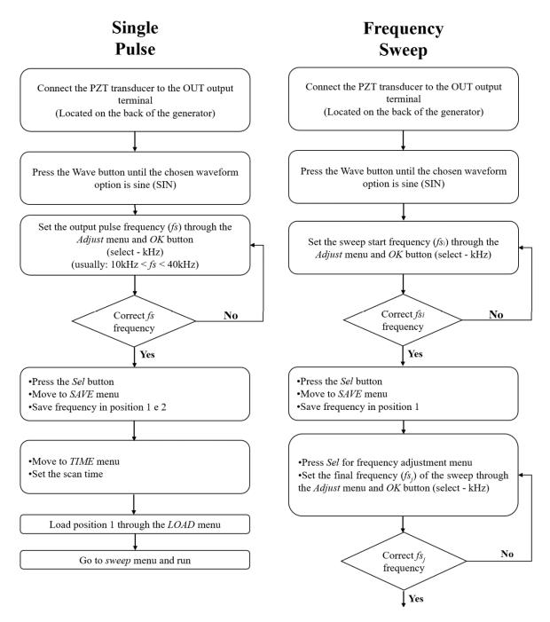
Figure 9: flowchart for setting up the UDB11008S wave generator.
