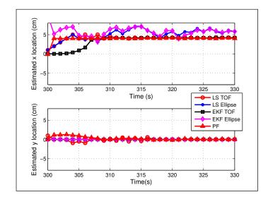
Figure 45: Least squares, extended Kalman filter, and particle filter convergence for both oneway ultrasonic pulse measurement models with the heating source located at (x = 4cm, y = 0cm)and an initial guess of (x = 0cm, y = 0cm).
