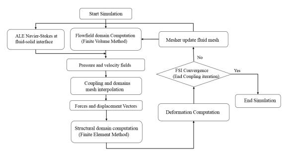
Figure 22: Fluid-structure coupling procedures
