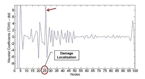
Figure 7 – DWT coefficients for V2E-2 beam using db5.
