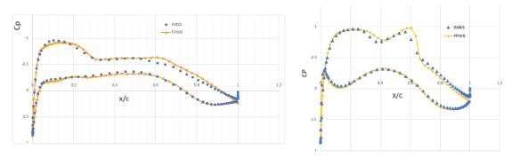
Figure 43: *Cp* distributions obtained with a RANS code and a full potential one for the ITA50ADV airliner. At left, station a 22% of semispan; right, station located at 50% of semispan ( $M_{\odot}$  = 0.775,  $\alpha$ =1.21°, Reynolds number of 15x10<sup>6</sup>)
