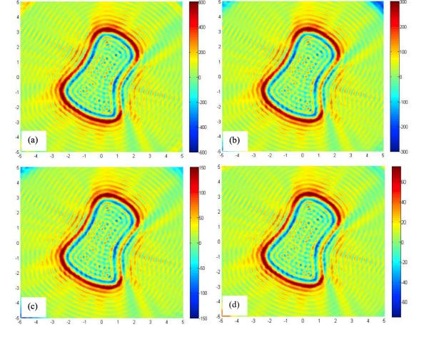
Figure 6: Identification of a single obstacle in an empty domain. Contour plots of  $D_T$  in terms of the distance to the receptors: (a)  $R_{meas}/D = 2.5$ , (b)  $R_{meas}/D = 5$ , (c)  $R_{meas}/D = 10$  and (d)  $R_{meas}/D = 20$ .
