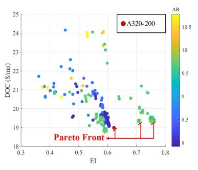
Figure 87: Optimization results with flutter constraint
