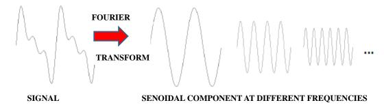
Figure 5 – Decomposition process of Fourier Transform (adapted from Misiti et al., 1997)
