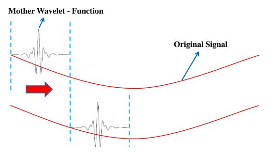
Figure 9 - Schematic calculus of wavelet coefficients (adapted from M Misiti et al., 1997).
