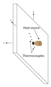
Figure 14: Illustration of flat plate with heat source and sensors (not drawn to scale).
