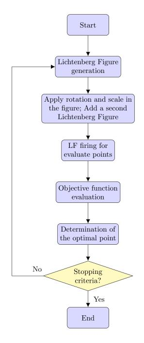
Figure 12: Lichtenberg Algorithm Flowchart.
