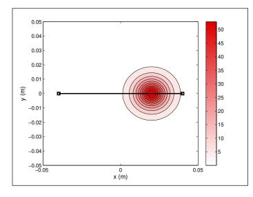
Figure 33: Temperature response at t = 320s with source located at (x = 2cm, y = 0cm).  $\theta_{avg} = 13.2K$  between sensors.
