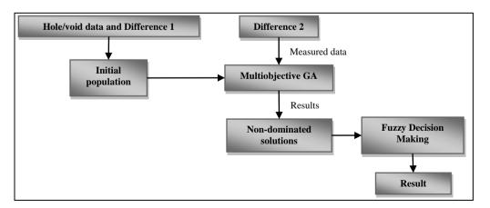
Figure 10: Flowchart for the optimization procedure using multiobjective genetic algorithm e fuzzy decision making.
