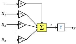
Figure 46: Artificial Neuron structure
