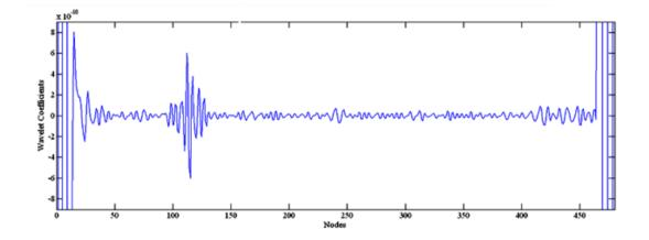
Figure 29 – Wavelet coefficients using bior3.7 of cantilever beam case with 0.5% of noise.
