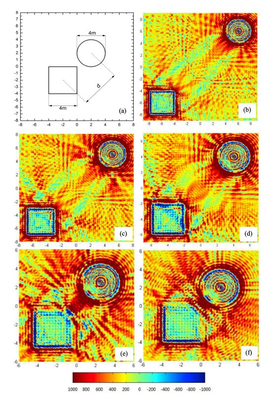
Figure 8: Identification of two obstacles in an empty domain. Contour plots of  $D_T$  in terms of the separation between the obstacles: (a) hidden obstacles, (b)  $d/r = 6\sqrt{2}$ , (c)  $d/r = 5\sqrt{2}$ , (d)  $d/r = 4\sqrt{2}$ , (e)  $d/r = 2.5\sqrt{2}$  and (f)  $d/r = 2\sqrt{2}$ . The same color scale is used in all the figures.
