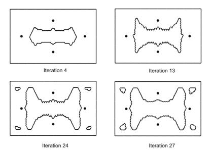
Figure 7: Topology evolution for the PCB
