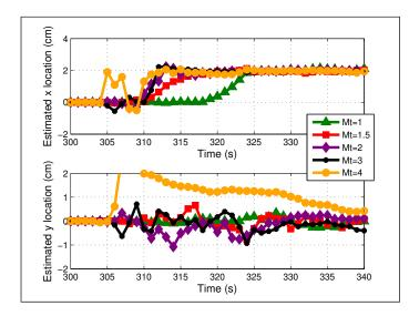
Figure 58: Adaptive extended Kalman filter convergence for a range of state model covariance gain values M, an initial state model covariance of  $Q_0 = 1-4m^2 \times I_2$ , and constant measurement covariance of  $R = 4-7 \times I_4$ . The heating source is located at (x = 2cm, y = 0cm) with an initial guess of (x = 0cm, y = 0cm).
