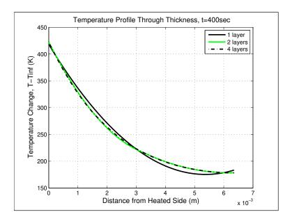
Figure 17: Number of mesh layers for best accuracy.
