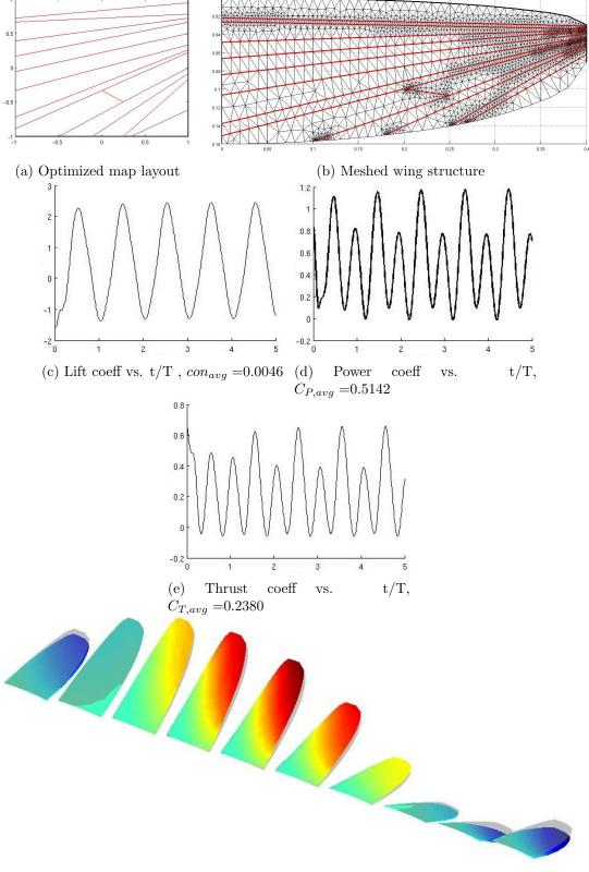
(f) Deformation of wing over a flapping cycle
