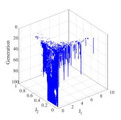
Figure 18: Pareto fronts for the 100 generations evaluated showing the convergence process.
