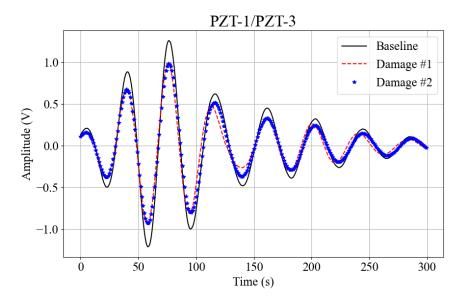
Figure 14: Averages of the characteristic wavelet scales of the states of the structure - Path PZT-1/PZT-3.
