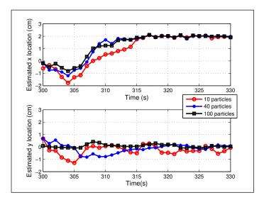
Figure 43: Particle filter convergence for selected numbers of particles with heating source located at (x = 2cm, y = 0cm) and an initial guess of (x = 0cm, y = 0cm).
