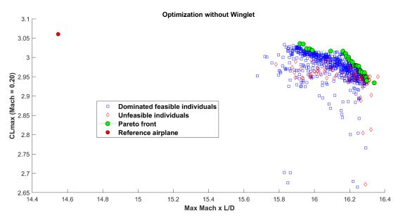
Figure 70: Optimization of wing airfoil geometry for a B757-200 similar aircraft
