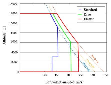
Figure 85: Flight envelope considering flutter speed constraints
