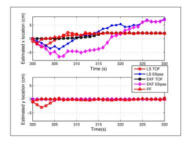
Figure 46: Least squares, extended Kalman filter, and particle filter convergence for both oneway ultrasonic pulse measurement models with the heating source located at (x = 6cm, y = 0cm)and an initial guess of (x = 0cm, y = 0cm).
