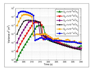
Figure 56: Adaptive extended Kalman filter variance  $(\sigma^2)$  from the state covariance matrix  $(\Sigma)$  for a range of starting state model covariance values  $(Q_0)$ , constant measurement covariance of  $R = 4-7 \times I_4$ , and  $M_t = 2$ . The heating source is located at (x = 2cm, y = 0cm) with an initial guess of (x = 0cm, y = 0cm).
