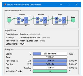
Figure 62: A main panel of the training/validation/test process with MATLAB® for the 120x120 network targeted to estimate the pitching moment coefficient
