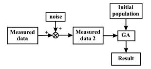
Figure 9: Flowchart for the analysis of the measurement error.
