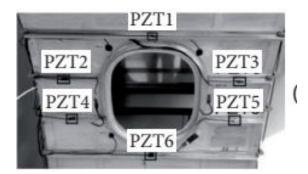
Figure 2: Aircraft aluminum window panel instrumented with six PZT patches (source: Maruo *et al*, 2015)
