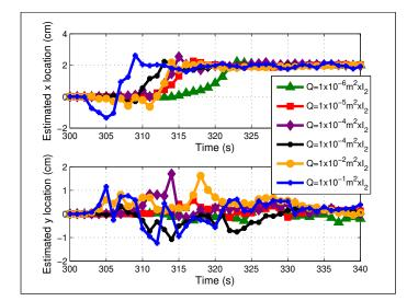
Figure 57: Adaptive extended Kalman filter convergence for a range of initial state model covariance values  $(Q_0)$ , constant measurement covariance of  $R = 4-7 \times I_4$ , and a state model covariance gain of M = 2. The heating source is located at (x = 2cm, y = 0cm) with an initial guess of (x = 0cm, y = 0cm).
