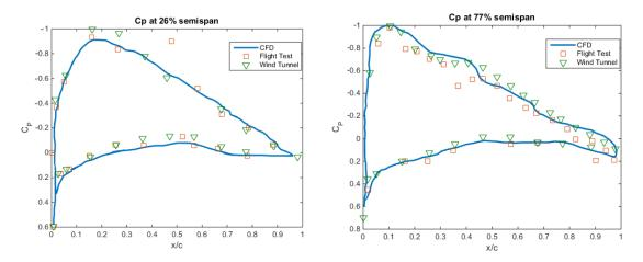
Figure 31: Calculated Cp distributions for the rigid model wing with no winglets compared with wind tunnel test and flight test data (Mach = 0.70,  $\alpha$  = 3.5°)
