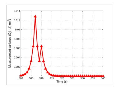
Figure 55: Adaptive extended Kalman measurement covariance  $(Q_t)$  values during convergence with  $Q_0 = 1 - 4m^2 \times I_2$ ,  $R = 4 - 7 \times I_4$ , and  $M_t = 2$ . The heating source is located at (x = 2cm, y = 0cm) with an initial guess of (x = 0cm, y = 0cm).
