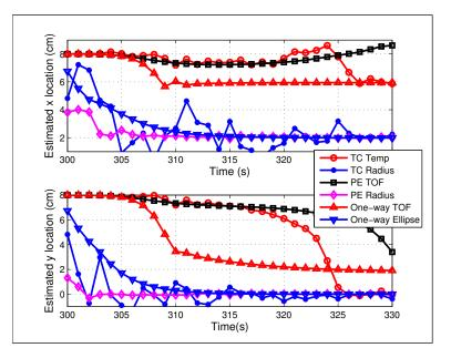
Figure 31: Extended Kalman filter convergence for all six measurement models with source at (2cm, 0cm) and initial guess of (8cm, 8cm).
