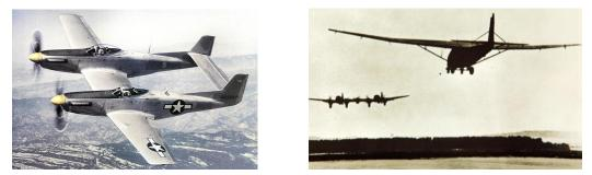
Figure 13: Dual-fuselage vintage aircraft. Left: Twin Mustang; Right: Heinkel He 111Z (Public domain photos)
