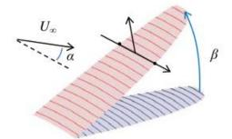
Figure 6: Characteristic angles and span-wise stations of the flapping wing with an attached coordinate system
