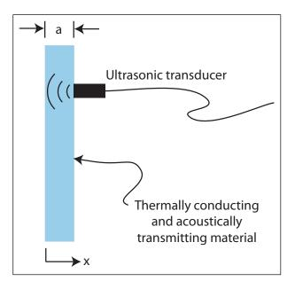
Figure 25: Ultrasonic pulse-echo technique.
