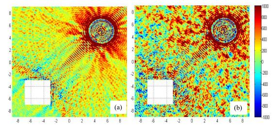
Figure 12: Assessment of the measuring error. Contour plots for the topological derivative results with (a) 10% and (b) 50% noise in the pressure values at the receptors.
