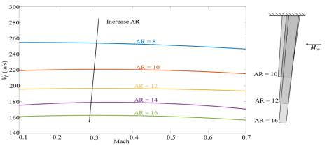
Figure 81: Influence of aspect ratio on flutter speed
