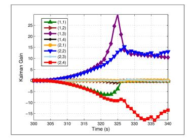
Figure 51: Kalman gain values during convergence for state model covariance of  $Q = 1-4m^2 \times I_2$ and measurement covariance of  $R = 4-7 \times I_4$ . The heating source is located at (x = 2cm, y = 0cm)with an initial guess of (x = 0cm, y = 0cm). Legend entries refer to the matrix element in the Kalman gain which is a  $2 \times 4$  matrix. Convergence (from Figure 50) is at 324s.
