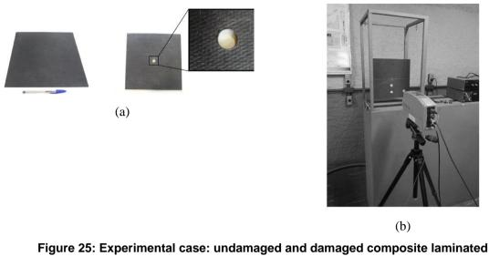
Figure 25: Experimental case: undamaged and damaged composite laminated plate (a) and Experimental setup of damage detection using contactless vibration measurement (b).
