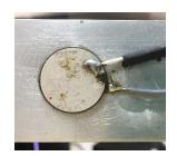
Figure 15: Specimen and PZT patch.
