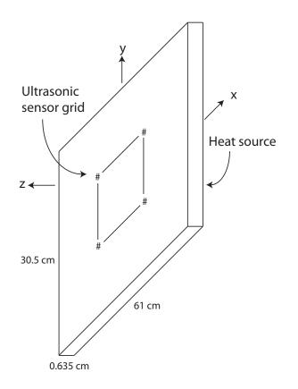
Figure 37: Ultrasonic sensor grid on the non-heated side of the plate with # symbols representing sensors and lines representing the ultrasonic pulse propagation paths between sensors (not drawn to scale).
