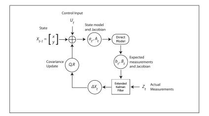
Figure 8: Parameter estimate update process using a the extended Kalman filter and a direct model.
