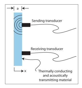
Figure 26: One-way ultrasonic pulse technique.
