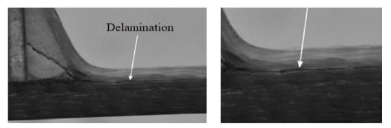
Figure 37: Composite laminated structure with delamination. Adapted from Heslehurst (2014).
