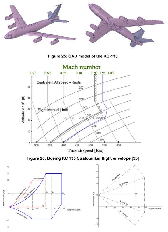
Figure 27: V-n diagram for the structural sizing of KC-135
