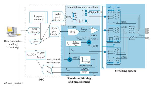
Figure 10: Architecture of a multiplexed sensor array for ISHM applications. Source: Maruo *et al* (2015).
