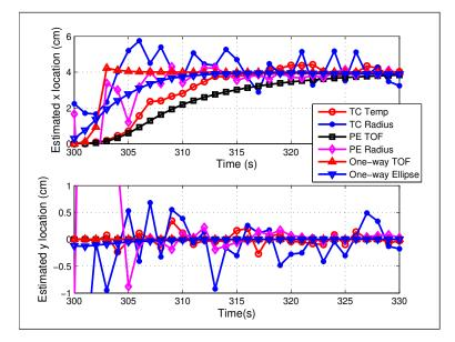
Figure 29: Extended Kalman filter convergence for all six measurement models with source at (4cm, 0cm) and initial guess of (0cm, 0cm).
