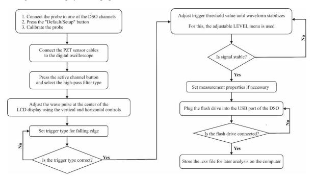
Figure 11: flowchart for B&K Precision Oscilloscope configuration.
