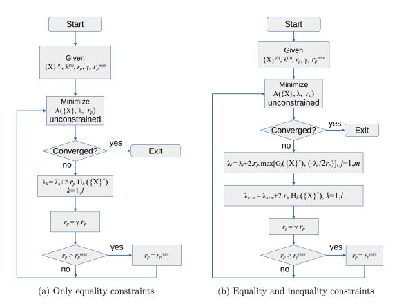
Figure 16: Augmented Lagrangian method for constrained optimization.
