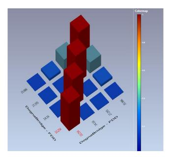
Figure 19 – AutoMAC correlation matrix of experimental mode shapes.
