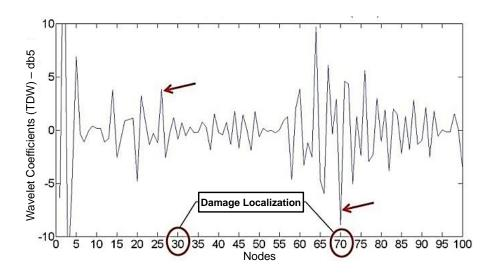
Figure 8 – DWT coefficients for V3E beam using db5.
