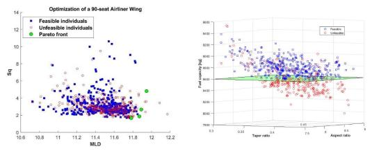
Figure 72: Simulation for the wing design of a 90-seat airliner. *Sq* is the square error that resulted after computing the difference between the prescribed and calculated *Cp* distributions at six stations along the wingspan
