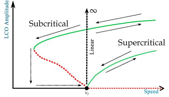
Figure 1: Generic flutter possibilities: linear, supercritical Hopf bifurcation, and subcritical Hopf situation; green color means stable behavior; red, unstable [5] [6]
