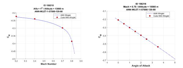
Figure 68: Comparison of pitch moment coefficient estimation for ID 156218 by the chosen ANN and that calculated by the full potential code. At left, variation with Mach number at a constant angle of attack; at right, variation with angle of attack at a Mach number of 0.70 and altitude of 10,000 m
