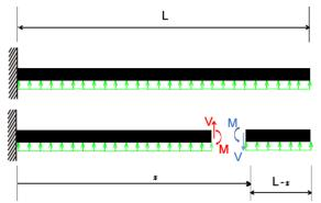
Figure 5: Internal reactions of a cantilever beam
