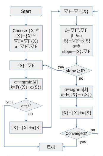
Figure 11: Flowchart with step-by-step description of Fletcher-Reeves Conjugate Direction method.
