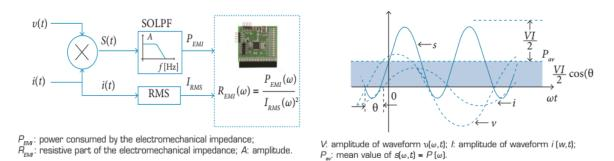
Figure 11: Topology to obtain the mean power  $P(\omega)$  (a). Equivalent waveforms (b). Source: Maruo *et al* (2015).
