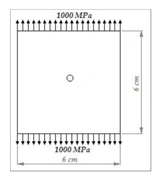
Figure 61: Plate model for the elastostatic problem.
