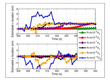
Figure 48: Extended Kalman filter convergence for a range of measurement covariance values (R) with constant state model covariance values of  $Q = 1-4m^2 \times I_2$ , the heating source located at (x = 2cm, y = 0cm), and an initial guess of (x = 0cm, y = 0cm).
