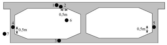
Figure 11. Location of the temperature sensors.
