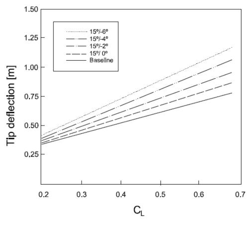
Figure 34: Wingtip deflection for some winglet configurations
