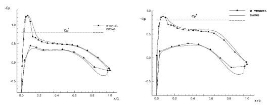
Figure 41: Pressure distributions for a station of the TRE planform at 22% (at left) and 66% (at right) of the wingspan. Mach = 0.700,  $\alpha$  = 0.365°
