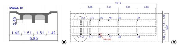
Figure 20 – Transversal cut view of damage D1(a) and localization of damage position by plan view(b).
