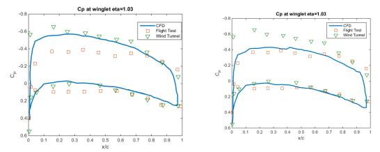
Figure 32: Calculated Cp distributions for the rigid and flexible models fitted with winglets. At left, Cp distribution in a winglet station for a CFD solution. At right, the FSI simulation results agree very well with flight test data (Mach = 0.70,  $\alpha = 3.5^{\circ}$ )
