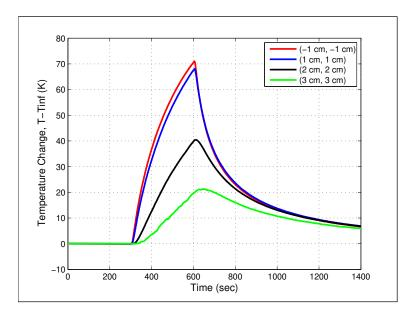
Figure 15: Temperature response on non-heated side of the plate at four sensor locations.
