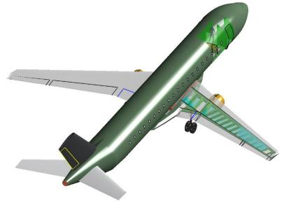
Figure 17: Example of wing layout for a 72-passenger airliner fitted with underwing engines
