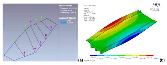
Figure 16 – Second frequency mode shapes of intact beam: (a) experimental (14.16Hz), (b) numerical (13.06Hz).
