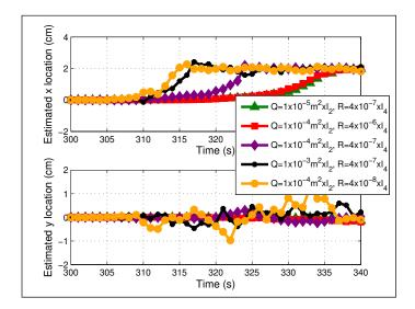
Figure 49: Extended Kalman filter convergence illustrating the correlation between the state model covariance matrix (Q) and the measurement covariance matrix (R). The heating source is located at (x = 2cm, y = 0cm) with an initial guess of (x = 0cm, y = 0cm).
