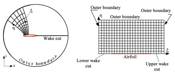
Figure 36: Coordinate transformation and mesh topology
