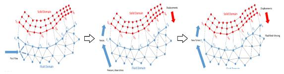
Figure 24: Mesh domains coupling and interpolation
