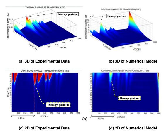
Figure 22 – Experimental and numerical comparation of CWT for damage D1 case.
