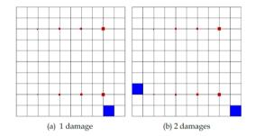
Figure 23: Result of damage identification in the delaminated plate considering 1 and 2 present damages (legend: damage detected, damages)
