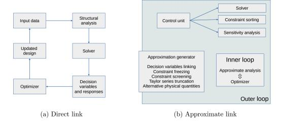
Figure 1: Comparison of the direct and approximate link between the Finite Element solver and the optimizer.
