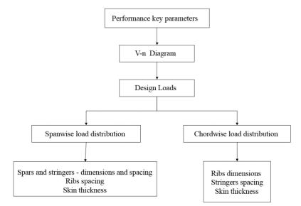
Figure 28: Calculation procedure of KC-135 wing structural elements
