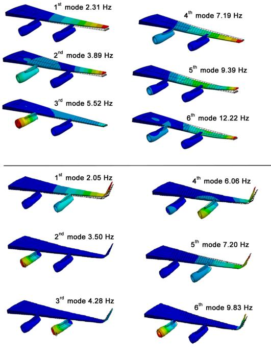
Figure 35: Mode shapes and frequencies of KC-135 wing with and without winglets
