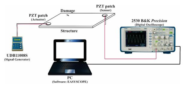
Figure 5: Low-cost Lamb Waves Experimental Setup.
