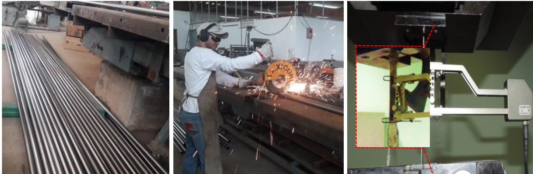
Barras de 6,0 metros com diâmetro de 38,0 mm.
