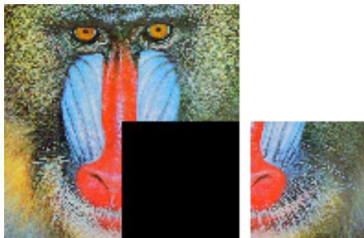
Figure 3.1: Example of input (left) and target (right) of the Intra prediction network used by [Minnen et al., 2017]. The input is the causal context obtained during the compression of the image, as it is a block based codec with raster scan ordering.
