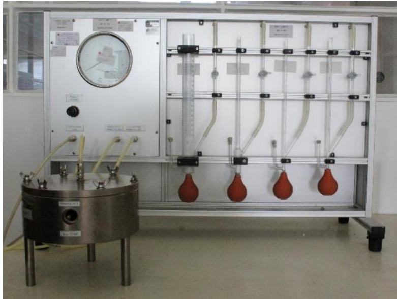
Figure 42 – CEMBUREAU air permeability equipment.
