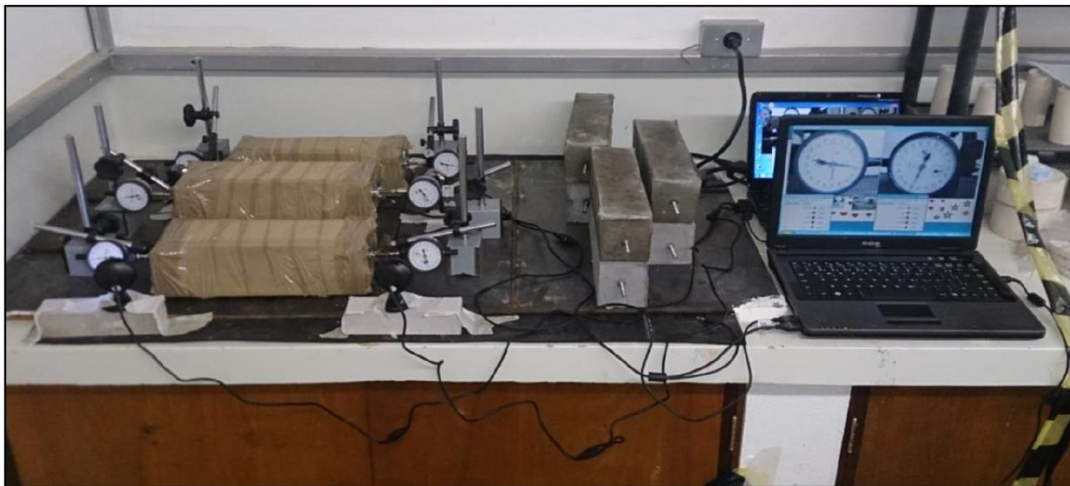
Figure 15 - Autogenous shrinkage test: (a) test setup scheme and (b) on going test.
