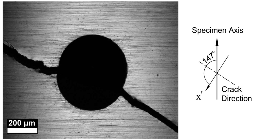
Figure 4.6 – Crack observed on the specimen S01 tested under square loading path ( \sigma_a = \tau_a = 105 MPa, N_f = 563,784 cycles).
