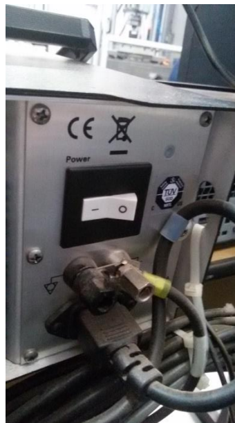
Figura B2: Interruptor do controlador MTS.
