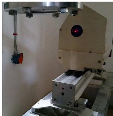
Figure A8: Atomizer coupled with the laser system
