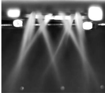
Figure A26: Liquid N<sub>2</sub>O discharged through vortex injector
