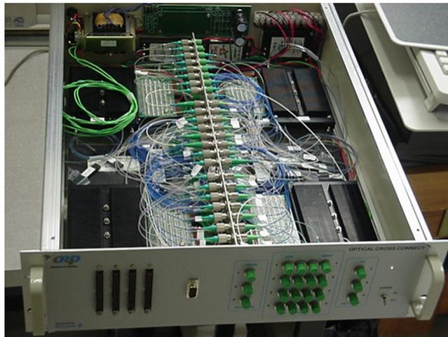
Figura 5.5 - *Optical cross-connect* (OXC) da rede OMEGA.
