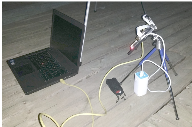
Figure 3.2: Lenovo Thinkpad notebook used to start the capture. The Nikon D5000 and the Raspberry Pi camera are controlled by a Raspberry Pi V2 minicomputer powered by a TP-Link 10400mAh Power Bank.
