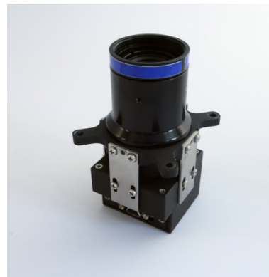
(b) ST400 star tracker: 48 \times 57 \times 89 mm, 280g.
