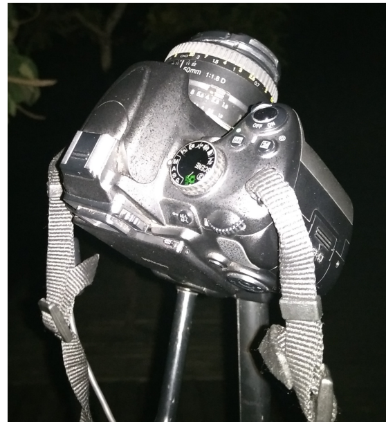
(b) Close up of the camera showing the 50mm D f/1.8 Nikon lens with the cap attached.
