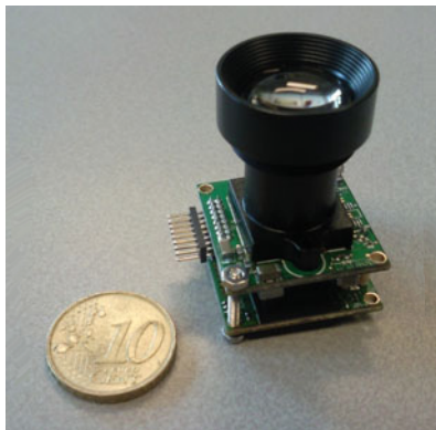
(a) ST200 star tracker: 30 \times 30 \times 38 mm, 40g
