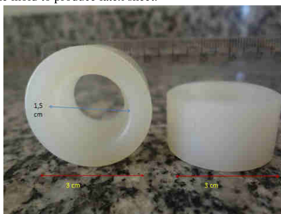
Figure 1. Image of holders made of tecnil to be attached to the glass base to produce latex lens sheet.
