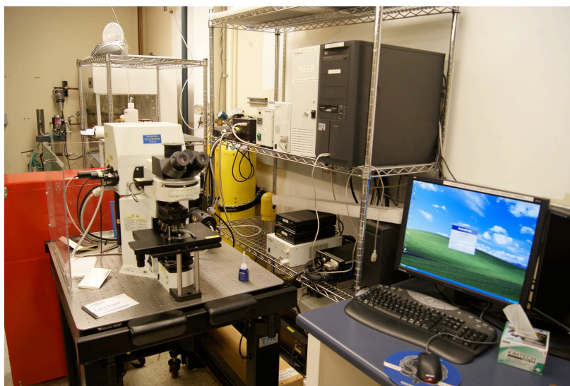
Figura 13: Imagem da bancada do Microscópio Confocal Olympus FluoView™ com varredura à Laser. (“Laboratory of Basic Science & Clinical Research, Trauma Division, UCSD/USA”).
