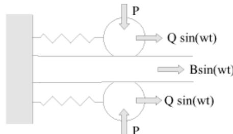
Figure 3. Schematic of experimental fretting fatigue configuration.
