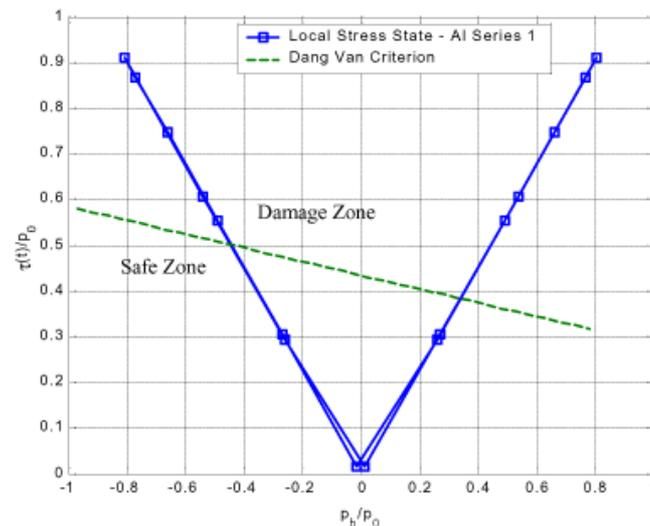
**Figure 6. History of local stress state and Dang Van fatigue criterion for AI series 1 data at  $(x,y)=(-1, 0)$ .**
