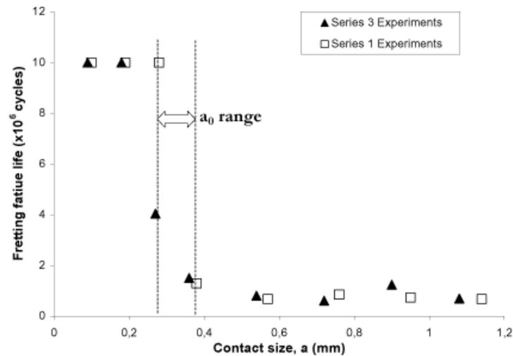
Figure 4. Results of Nowell's (1988) fretting fatigue experiments: variation of life with contact size.
