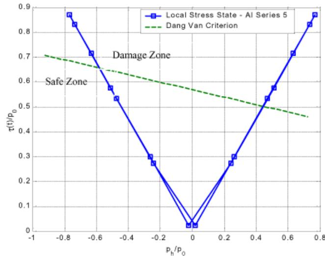
Figure 7. History of local stress state and Dang Van fatigue criterion for Al series 5 data at  $(x,y)=(-1.0, 0)$ .
