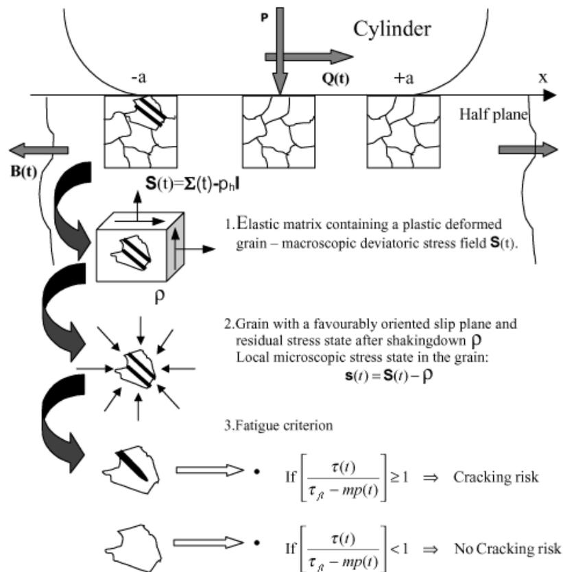
Figure 2. Different steps of the high cycle fatigue criterion proposed by Dang Van et al. (1989).
