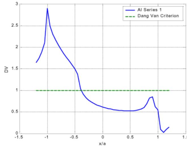
**Figure 5. Surface variation of the Dang Van cracking risk parameter DV for AI series 1.**
