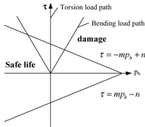
Figure 1.  $\tau \times \rho_h$  plane showing the torsion and bending load paths.
