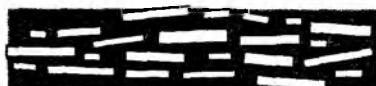
Fig. 1: 2D view of the sedimented samples' geometry. The mesoporous space is denoted by the gray shading. The clay particles have their silica sheets oriented along the horizontal direction, on average. The RMS deviation for the alignment of individual particles from this mean orientation is between 15 and 16.5° 11) .
