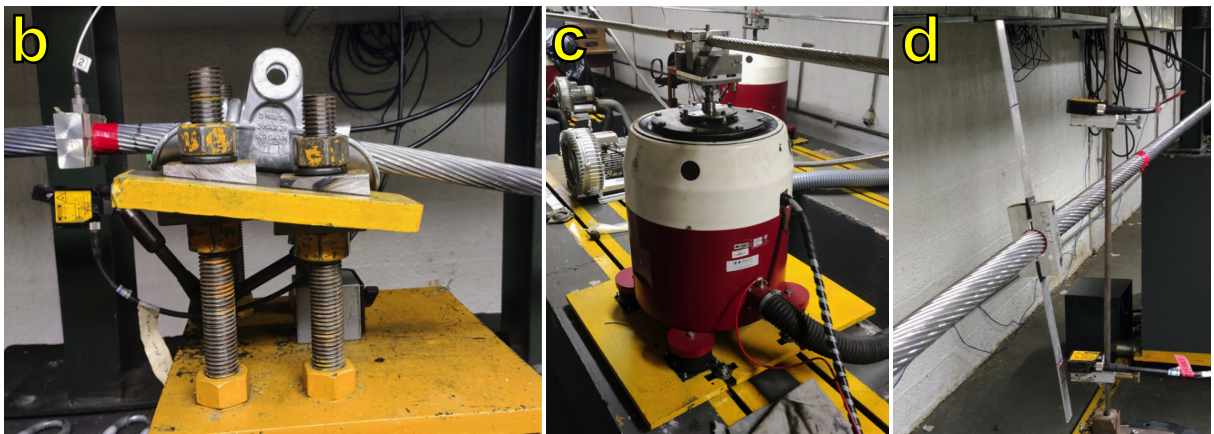
Figure 2.16: Resonant fatigue test benches: (a) schematic overview, (b) conductor/clamp assembly, (c) electronic shaker and (d) rotation sensor.
